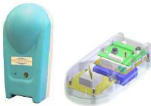
Figure 2. View of the dosimeter used in this study and its internal structure.
