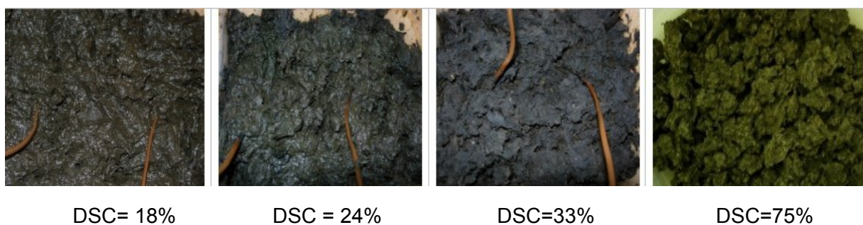
Figure 2. 8 Deformation and shrinkage due to water content evolution
