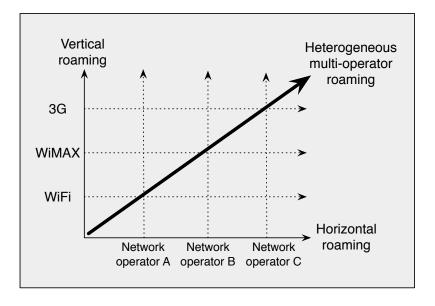
Figure 3.17: Roaming in Heterogeneous Multi-Operator Environments
