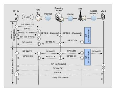
Figure 5.13: Roaming-SIP Signaling Exchange
