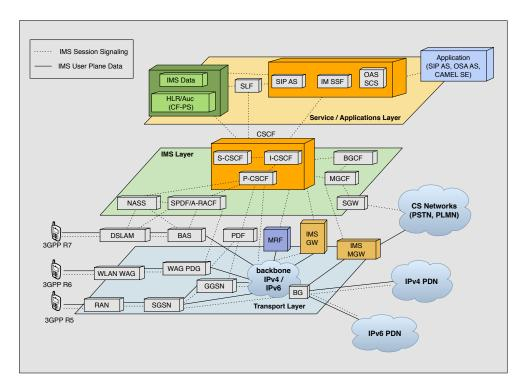
Figure 3.18: SIP integration in current wireless architectures
