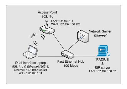
Figure C.1: Testbed for Access Control mechanism
