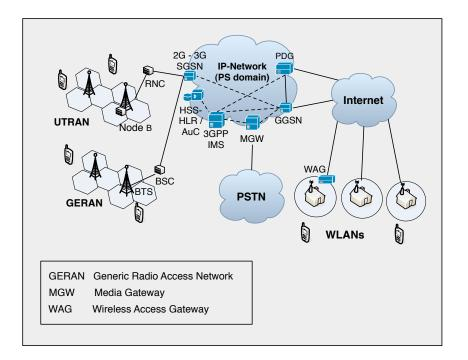
two elements: the IMS and the PDG (Packet Data Gateway), see Figure 3.4.
