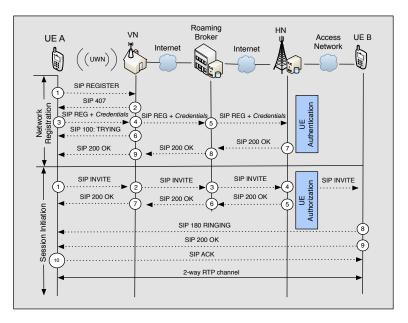
Figure 4.4: SIP-based Roaming Signaling
