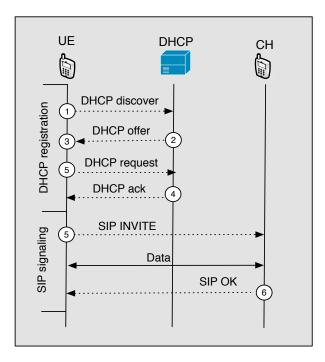
Figure 3.16: Signaling for UTMS-to-WLAN handover
