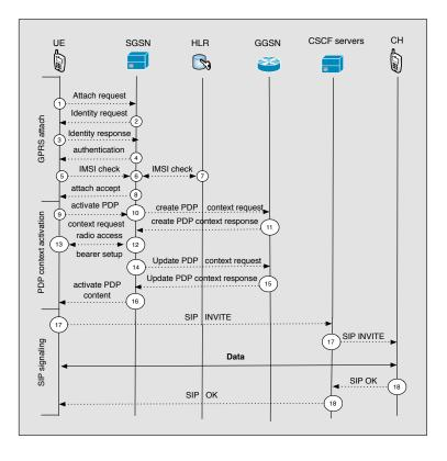
Figure 3.15: Signaling for WLAN-to-UMTS handover
