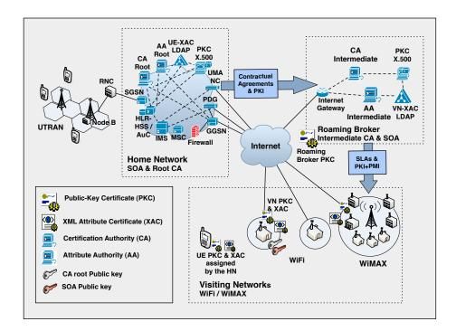
Figure 5.11: SIP & PMI-based Roaming Architecture
