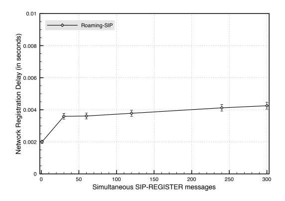
Figure 4.13: Network Registration Delay (in the HN)
