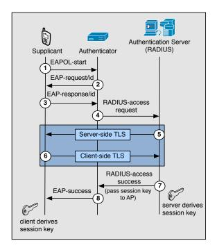
Figure 5.5: Message Flow of EAP-TLS
