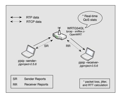
Figure B.4: RTCP statistics with the WRT54GL
