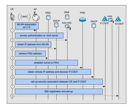
Figure 3.5: IMS registration through WLAN
