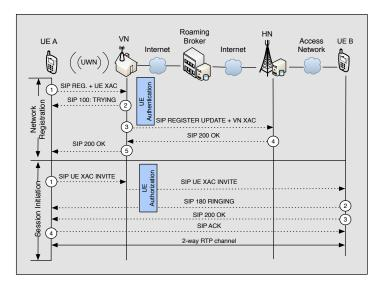
Figure 5.14: SIPXACs Signaling Exchange
