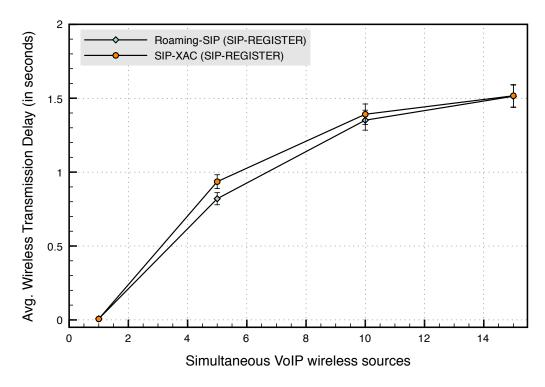
Figure 5.17: Avg. Wireless Transmission Delay for Network Registration
