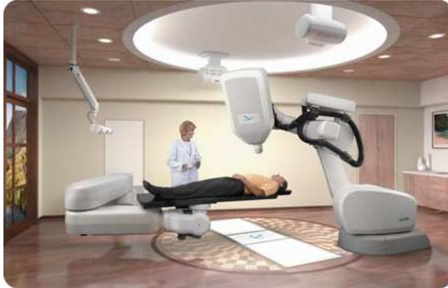
Figure 2.13: The CyberKnife combines continuous image-guidance technology with a compact linear accelerator that has the flexibility to move in three dimensions according to the treatment plan ([www.accuray.com](http://www.accuray.com)).
