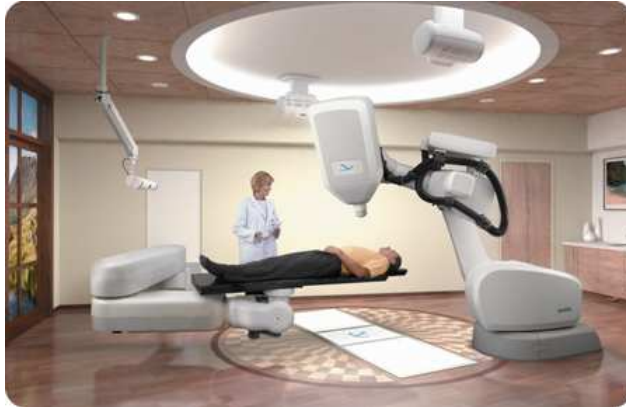
Figure 2.13: The CyberKnife combines continuous image-guidance technology with a compact linear accelerator that has the flexibility to move in three dimensions according to the treatment plan ( www accuray.com ).
