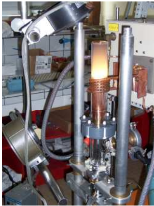
Figure II.2-a: Four à induction (INSA / Rennes)
