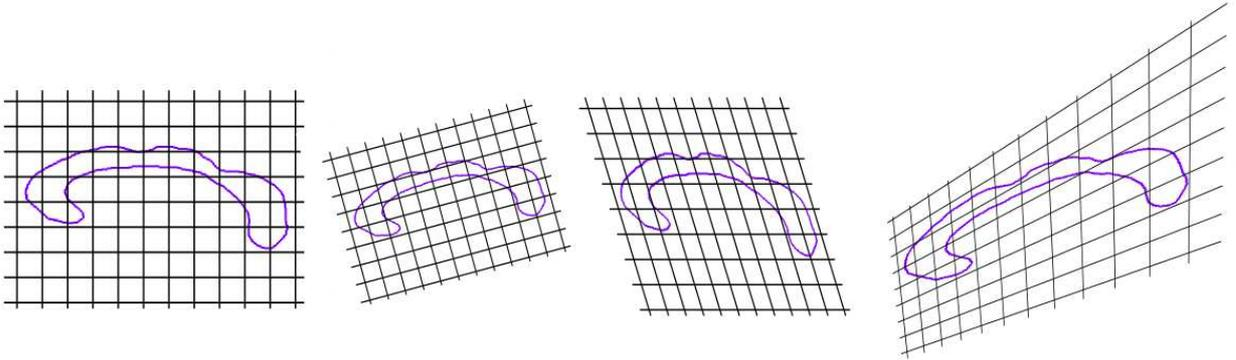
Fig. 2.5: Classic global transformations. From left to right, identity, rotation+scaling, affine, perspective transformation
