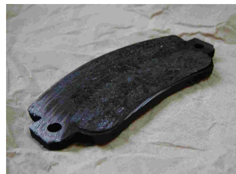
FIG. 1.18: Usure excessive des plaquettes
