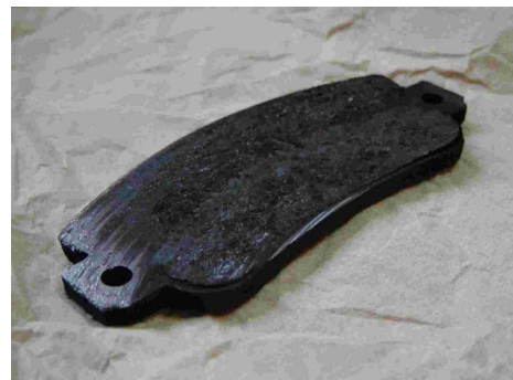
FIG. 1.18: Usure excessive des plaquettes
