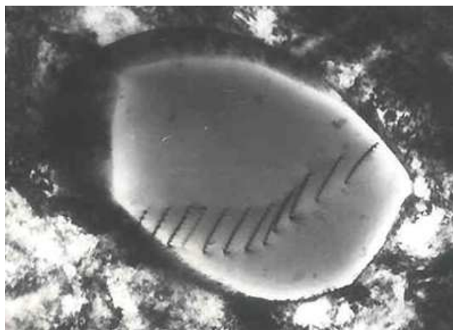
FIG. 2.1 – Dislocations in stainless steel.
