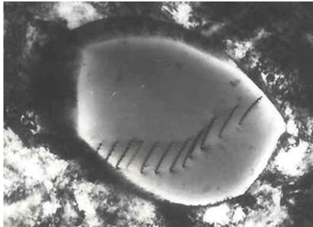
FIG. 2.1 – Dislocations in stainless steel.
