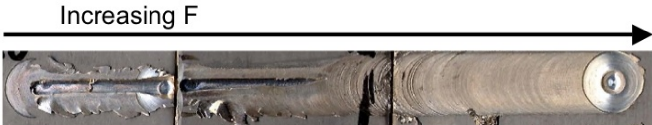
Figure 4.9: Digital image showing the influence of the applied pressure (from 5.2 to 6.5 kN) on the weld quality for AZ31 FSW ( W = 1000 RPM, V = 200 mm/min).
