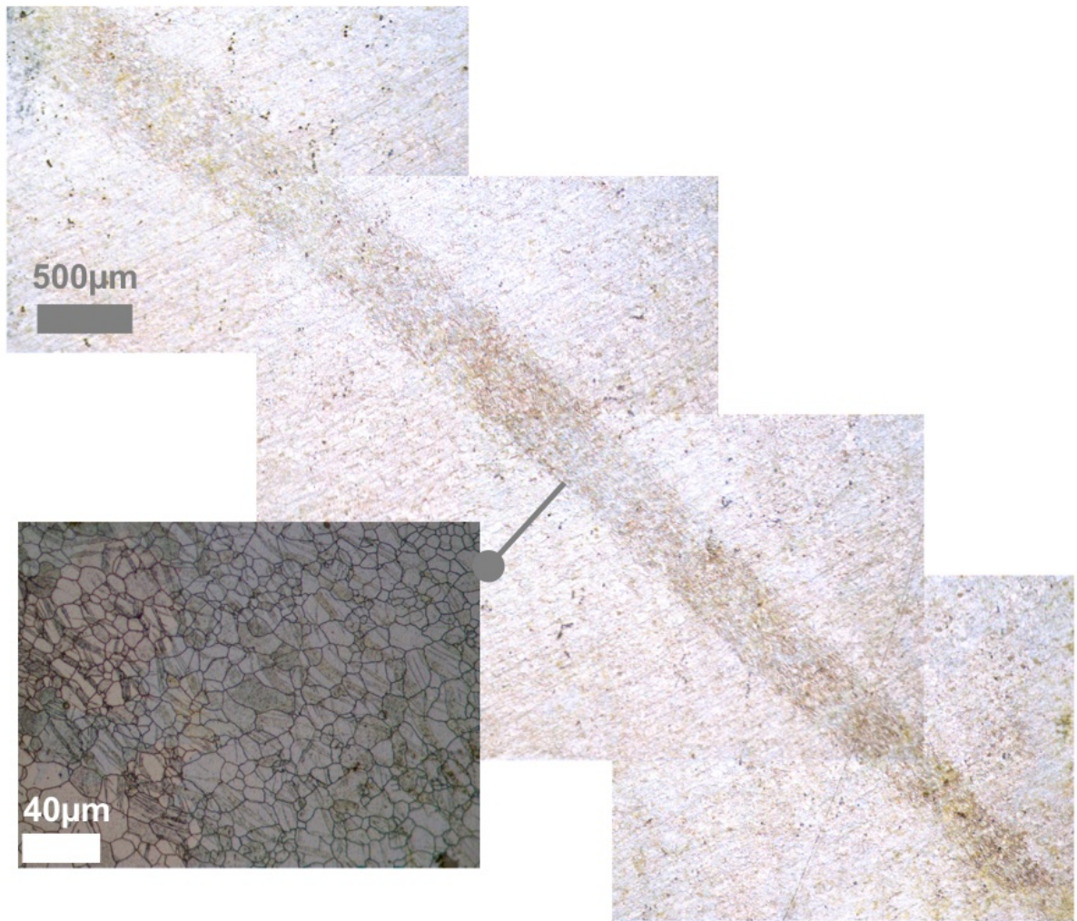
Figure 5.13: Optical micrograph of one shear band in FSW (13 mm shoulder diameter, W = 1000 RPM, V = 200 mm/min).
