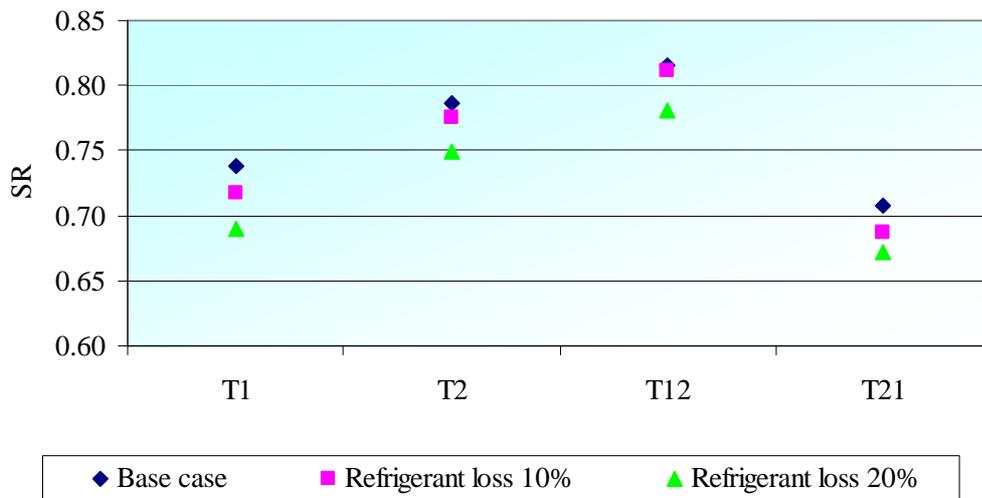
Figure 19: Sensible to total heat transfer ratio for the base case and for refrigerant leaks
