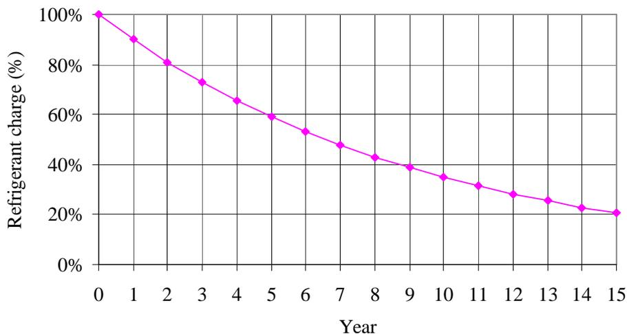
Figure 98: Refrigerant charge evolution with a yearly leak rate of 10 %
