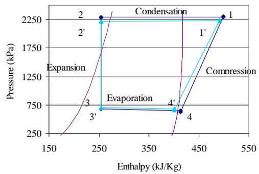
— R22 saturation —●— Reference case —▲— Compressor efficiency -13 %
