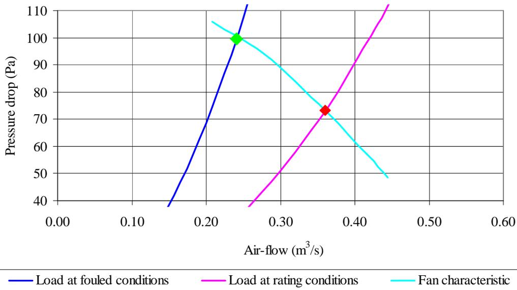
Figure 14: Fan characteristic and pressure drop for rating and fouled conditions at the evaporator
