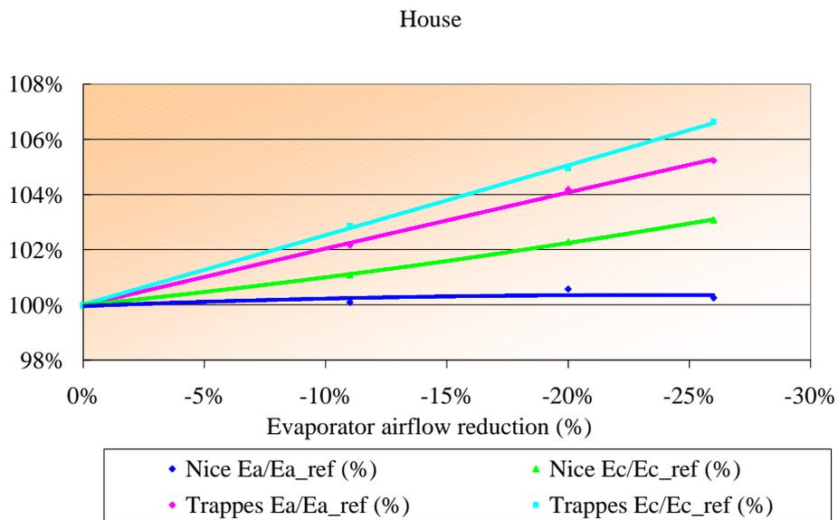
Figure 135: Effect on the cooling energy and the annual energy consumption for a house in Nice and Trappes for filter fouling
