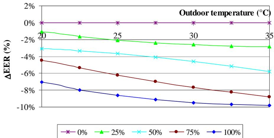
Figure 78: Effect on the efficiency for the tandem for increased condenser pressure drop
