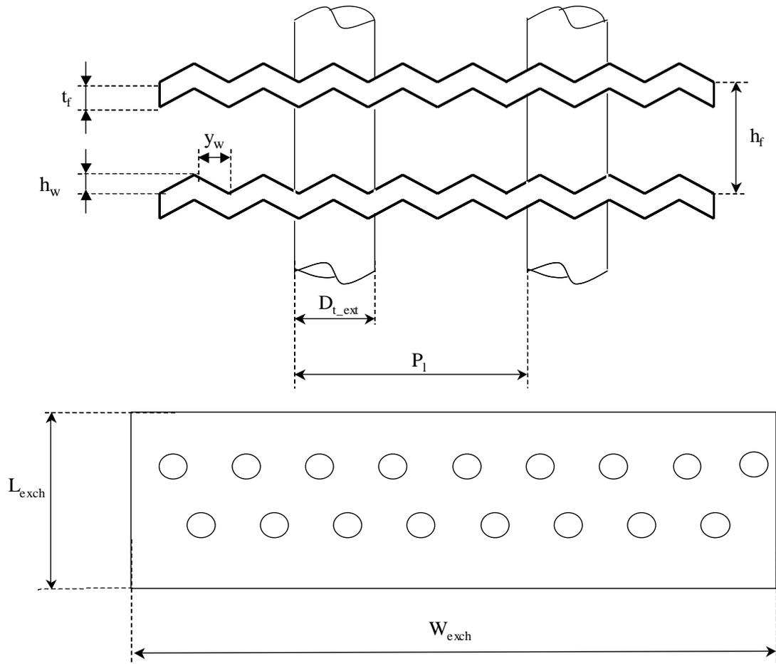
Figure 100: Geometric parameters of the heat exchanger
