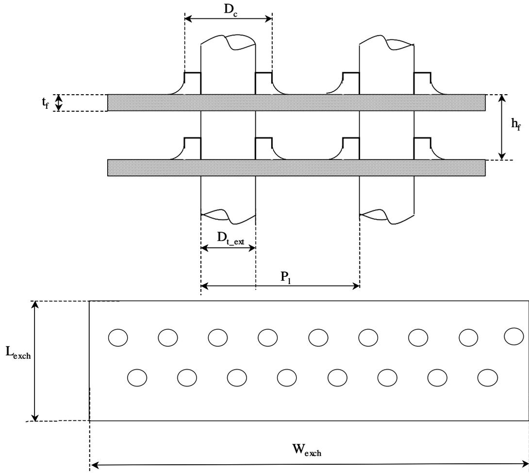
Figure 9: Geometric parameters of the heat exchangers
