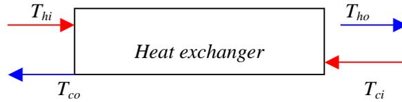
Figure 62: Heat exchanger hot and cold fluids scheme
