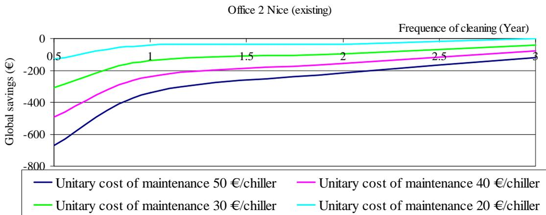
Figure 156: Global savings for regular condenser cleaning for office building 2 for an existing (fouled) system
