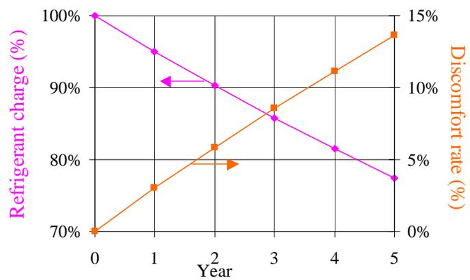
Figure 148: Refrigerant charge, capacity and comfort evolution for an office in Nice
