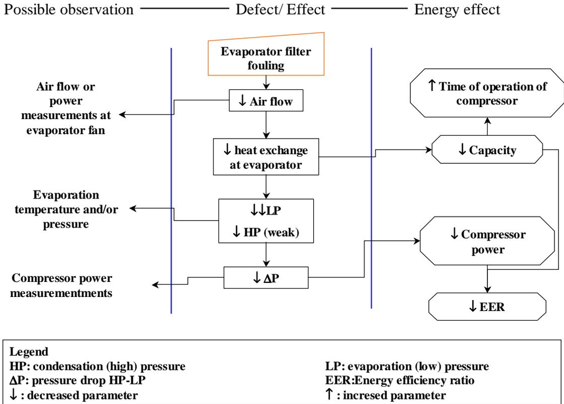
Figure 13: Tree representation of evaporator filter fouling consequences and possible measurement parameters
