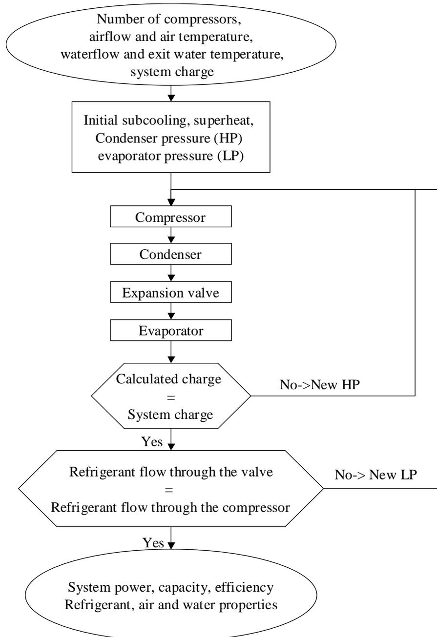
Figure 65: Model scheme for convergence on refrigerant charge
