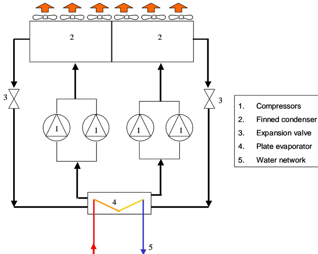
Figure 51: Scheme of components of the original chiller
