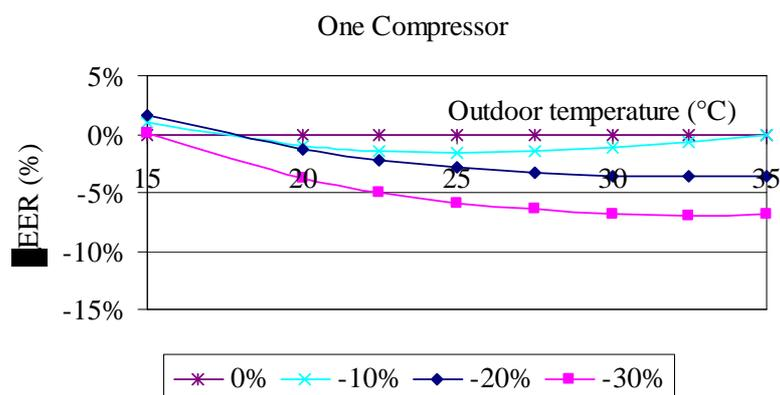
Figure 82: Efficiency variation with non-condensable in the condenser (one operating compressor)
