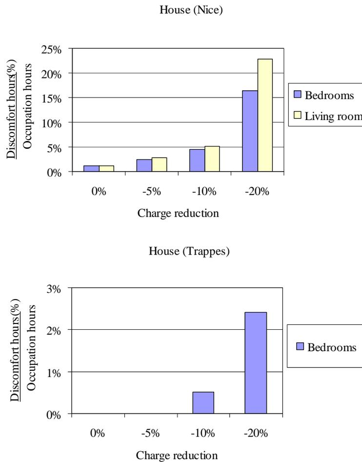
Figure 131: Subsequent discomfort for reduced refrigerant charges for a house in Nice and Trappes
