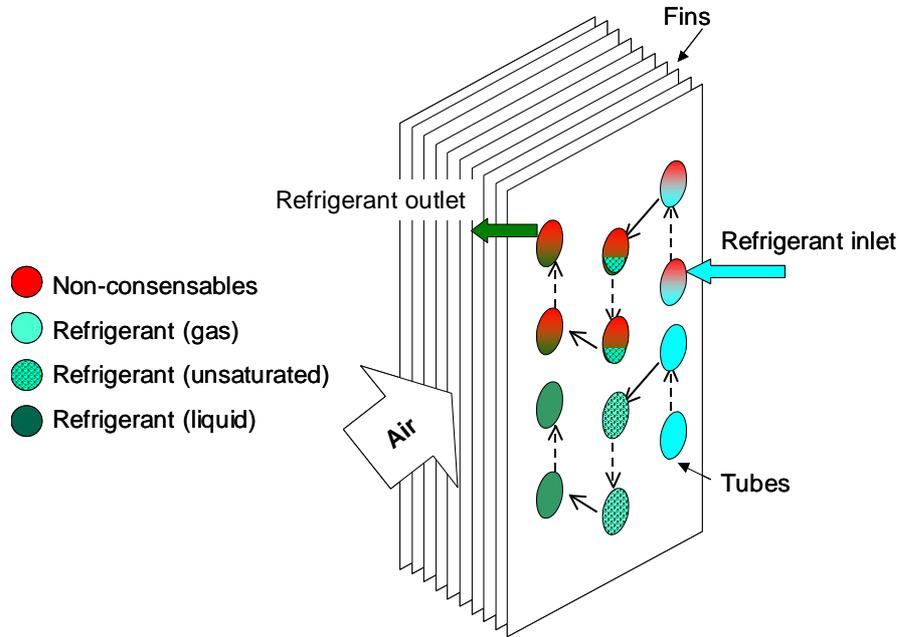
Figure 55: Non-condensable gases accumulation in the condenser
