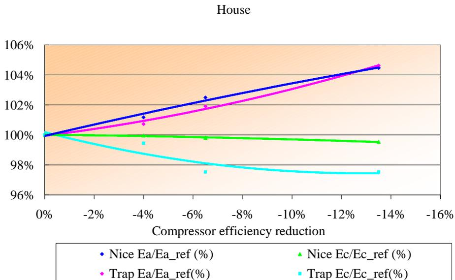
Figure 144: Effect on the cooling energy and the annual energy consumption for an office building in
