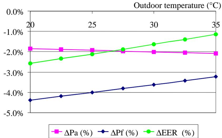
Figure 72: Performance effect of 10 % refrigerant leak (two compressors)
