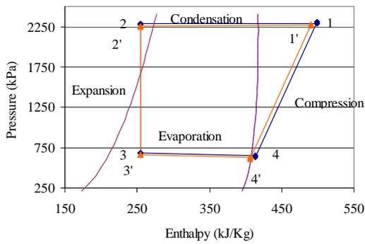
— R22 saturation —●— Reference case —▲— Evaporator airflow -11 %
