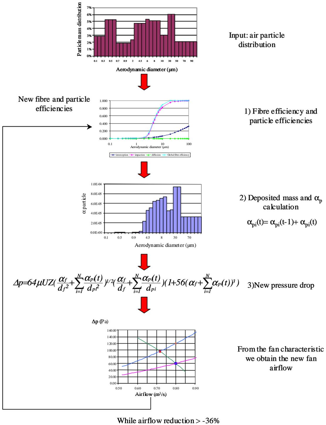
Figure 118: Scheme of the program for filter fouling
