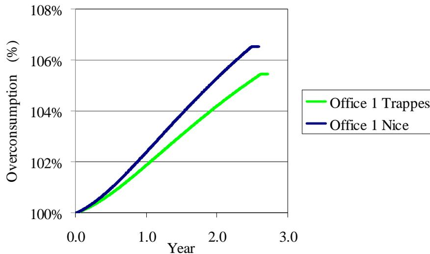
Figure 111: Overconsumption evolution with fouling and with maintenance for office 1 in Trappes
