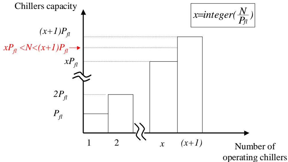
Figure 89: Scheme of the control of start of the chillers for the cooling load  $N$
