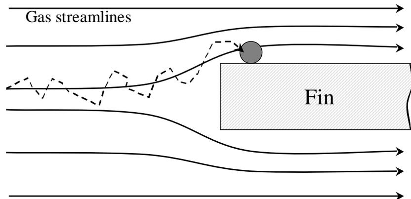
Figure 103: Particle deposition due to Brownian turbulence
