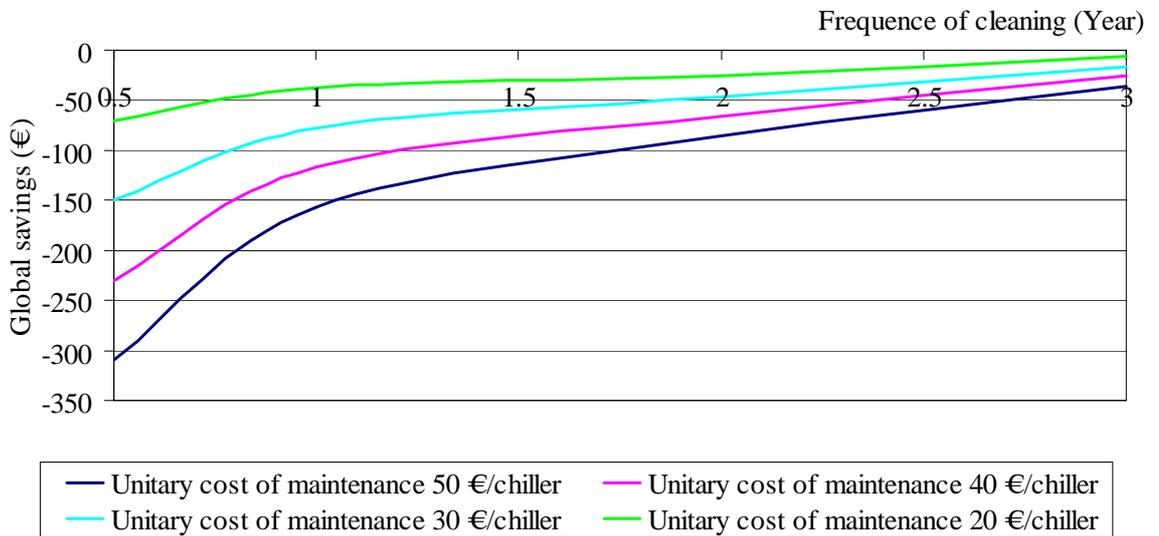
Figure 158: Global savings for regular condenser cleaning for office building 3 for a new (clean) system
