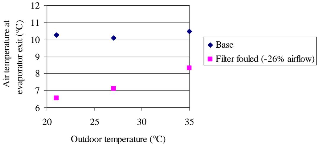
Figure 29: Air temperature at the evaporator exit with clean and fouled filter.
