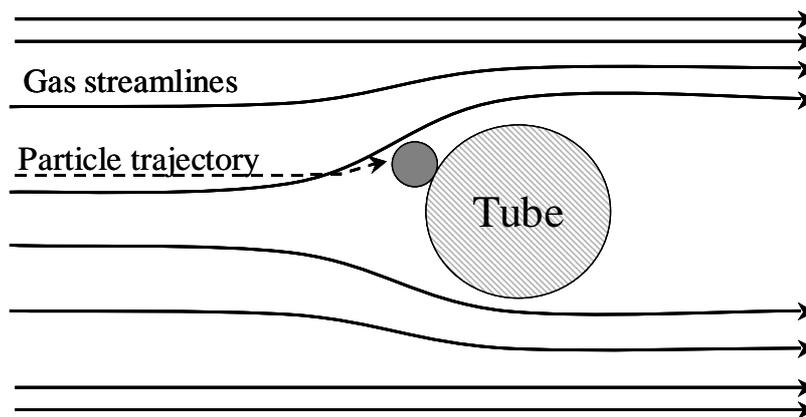
Figure 102: Particle deposition due impaction on tubes
