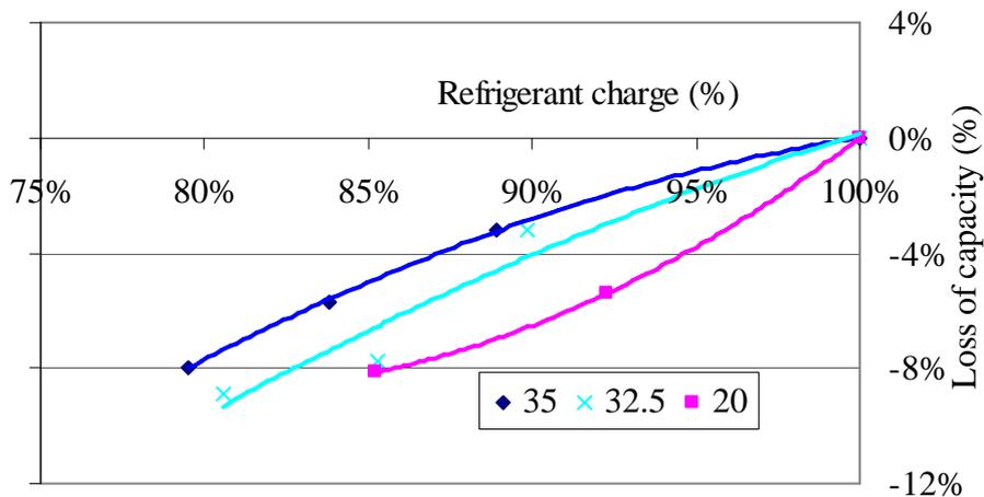
Figure 71: Capacity losses for different refrigerant charge levels
