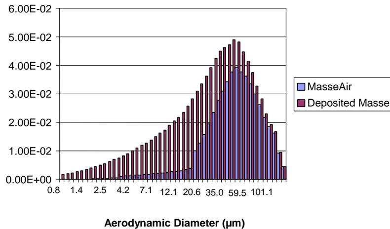
Figure 108: Mass distributions of air particles and deposited particles for SAE dust.
