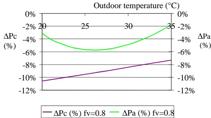
Figure 84: Influence of the clogged valve factor for different outdoor temperature values on the capacity ( $P_c$ ) and the absorbed power ( $P_a$ )
