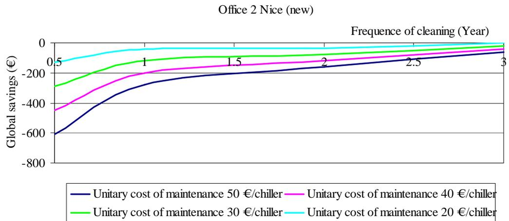
Figure 155: Global savings for regular condenser cleaning for office building 2 for a new (clean) system
