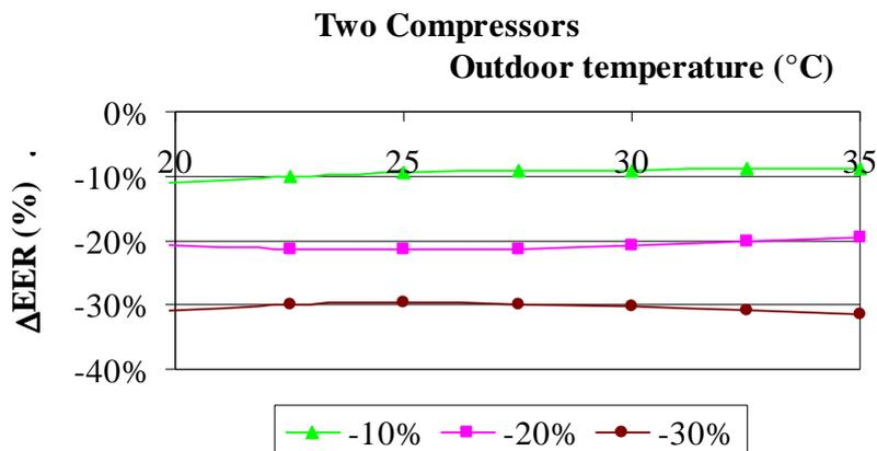
Figure 85: EER effect for worn compressor
