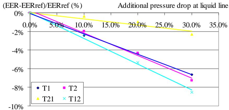
Figure 35: Effect of additional pressure drop in the liquid line on the EER.
