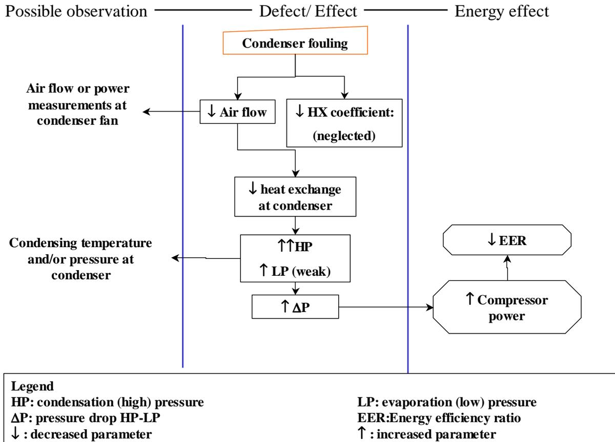
Figure 8: Tree representation of condenser fouling consequences and possible measurement parameters
