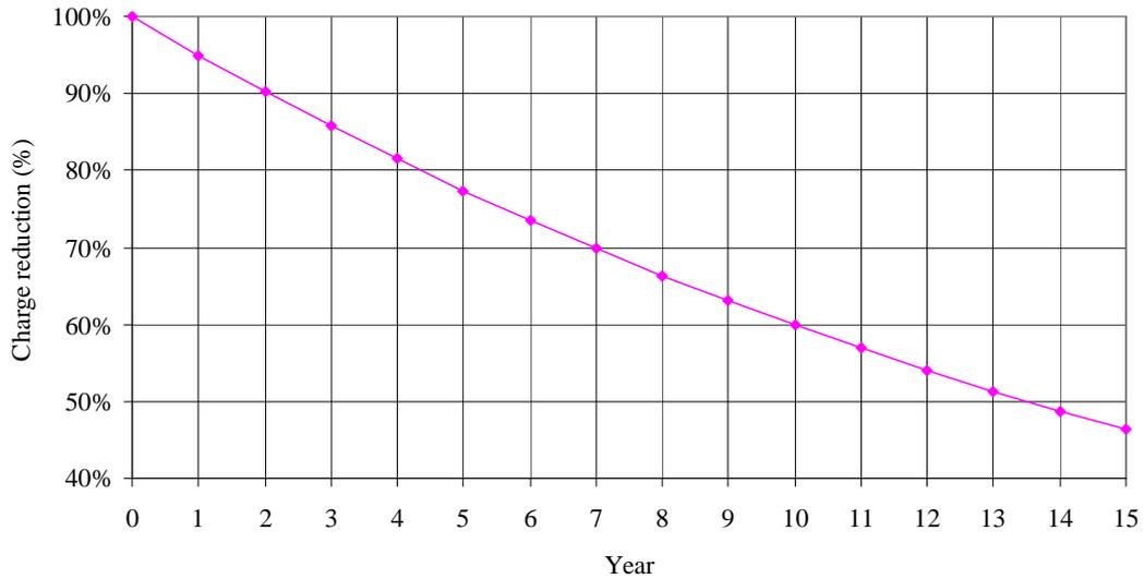
Figure 96: Charge evolution with an annual leak rate of 5 %
