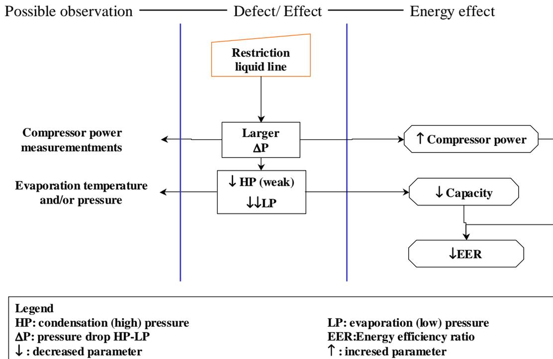
Figure 15: Tree representation of restriction in the liquid line consequences and possible measurement parameters
