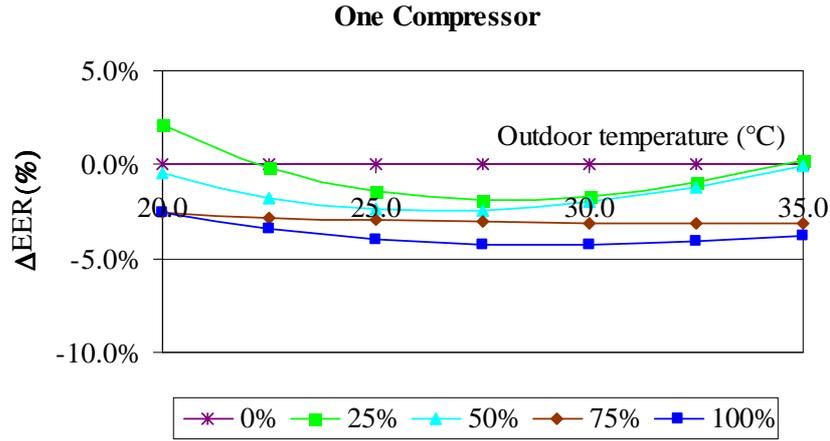
Figure 79: Effect on the efficiency for the one operating compressor for increased condenser pressure drop
