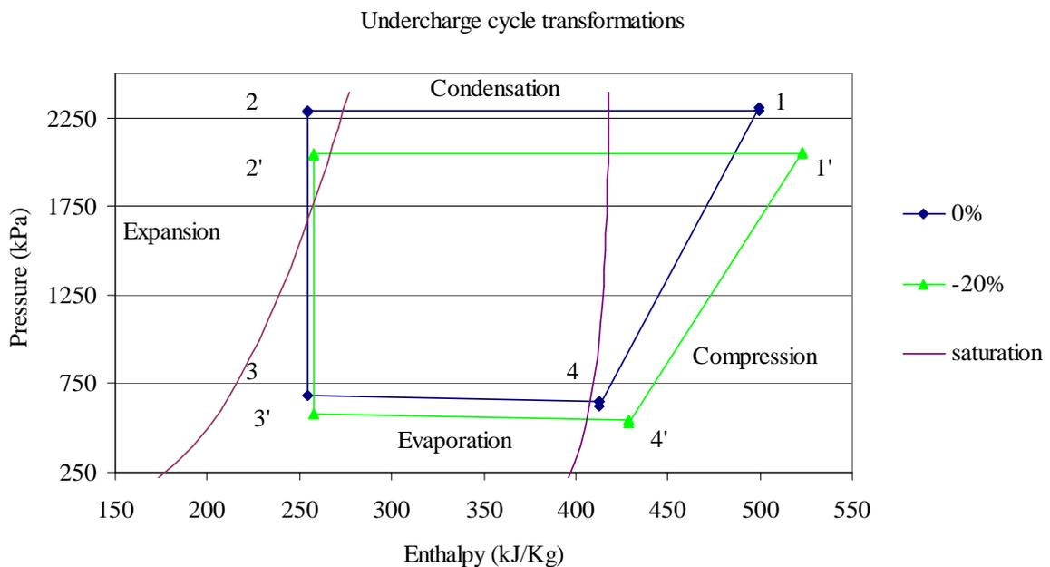
Figure 17: Thermodynamic R22 cycle modification for undercharged system
