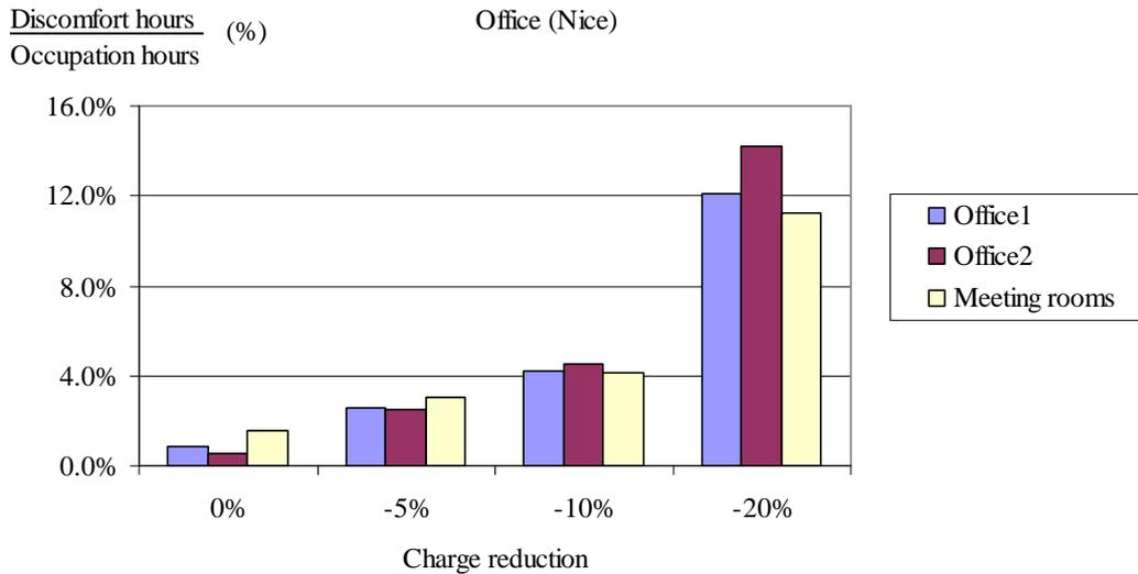
Figure 41: Subsequent discomfort for reduced refrigerant charges for an office building in Nice
