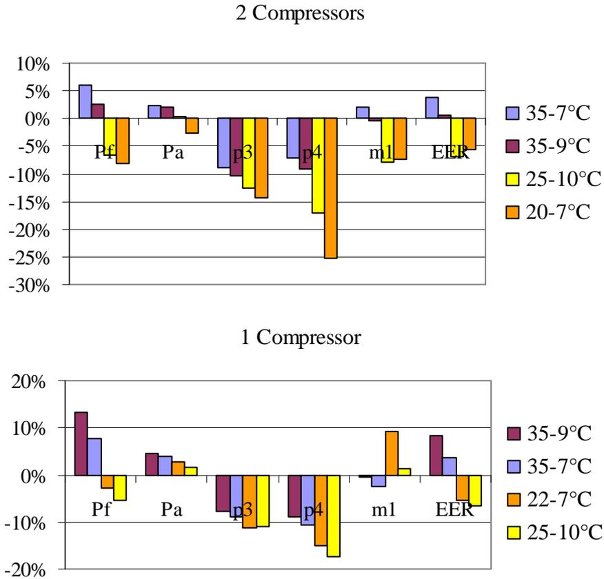
Figure 69: Errors of the model for one and two operating compressors comparing to experimental data
