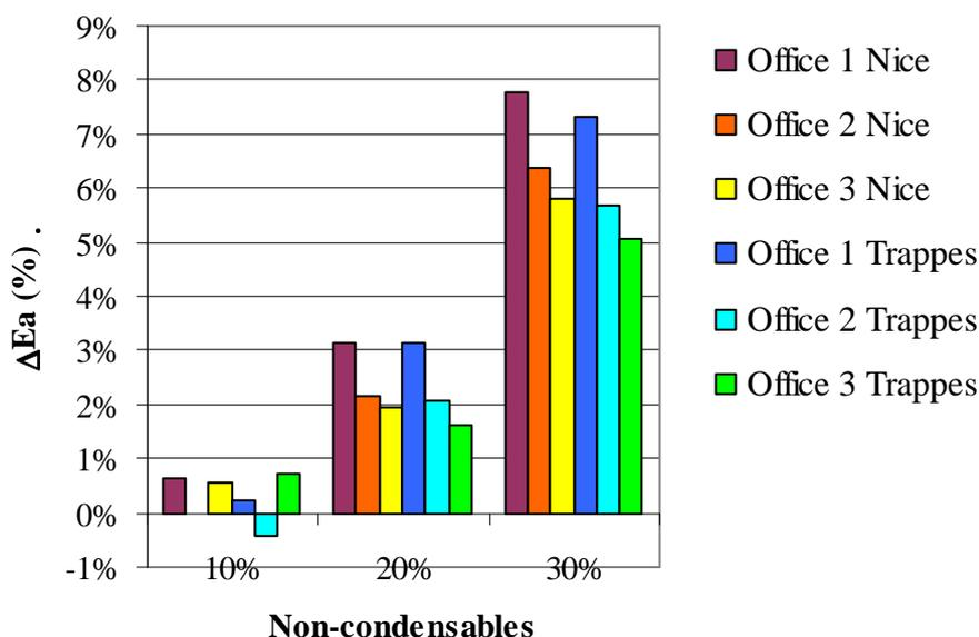
Figure 92: Condenser fouling effect on the seasonal consumption for the three office buildings and two analysed weather conditions
