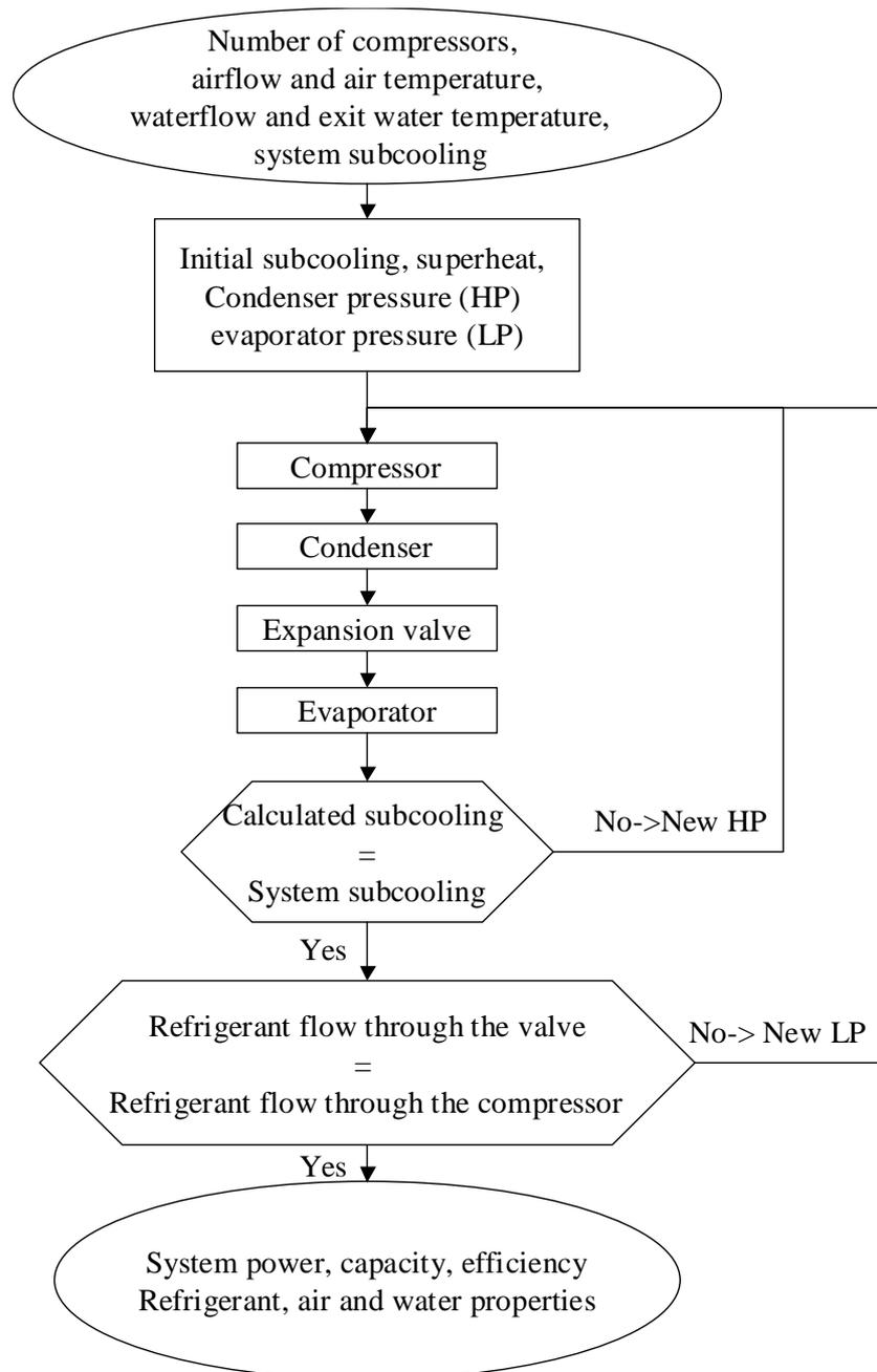
Figure 64: Model scheme for convergence on subcooling
