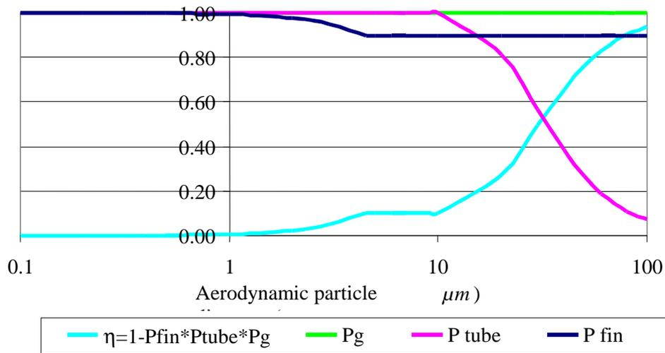
Figure 107: Deposition fraction of the heat exchanger as a function of the aerodynamic particle diameter
