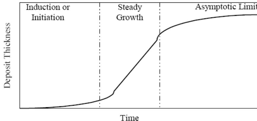
Figure 7: Asymptotic fouling modelled by Bott [Bott 1995]
