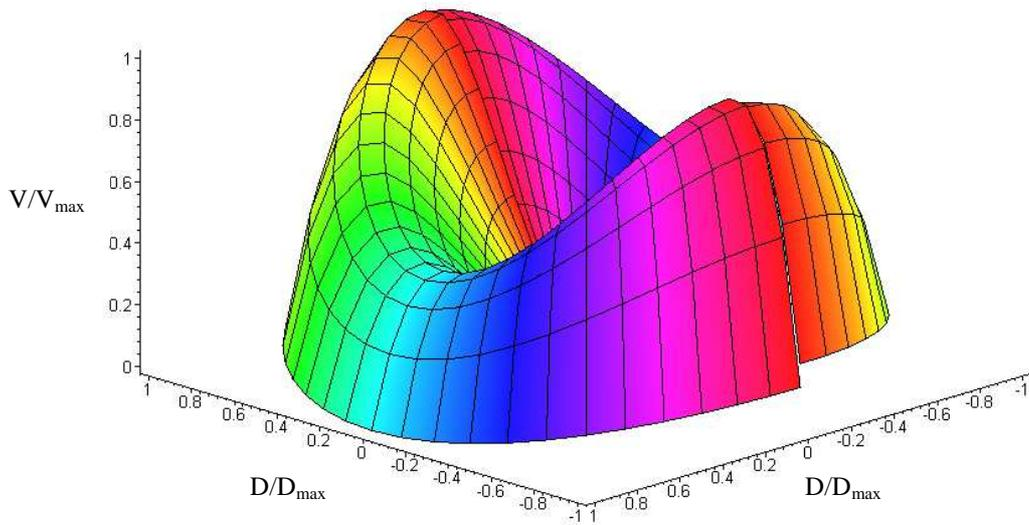
Figure 24: Normalised condenser fan airflow velocity profile
