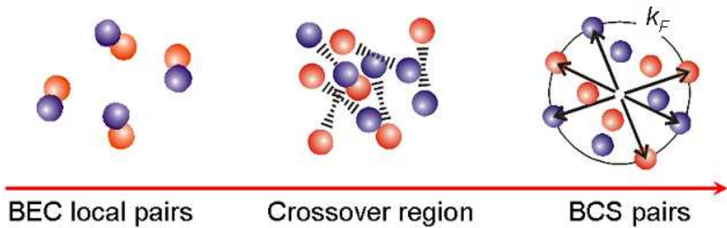
Figure 3.5: Superfluidity with zero total momentum pairing. This figure shows how the pairing changes across the BEC-BCS crossover. The left panel shows the BEC superfluid of the effective local bosons. The right panel shows the weak-coupling limit with the formation of the BCS superfluid with pairing at large distances. The middle panel shows the unitary regime with pairing at intermediate distances.
