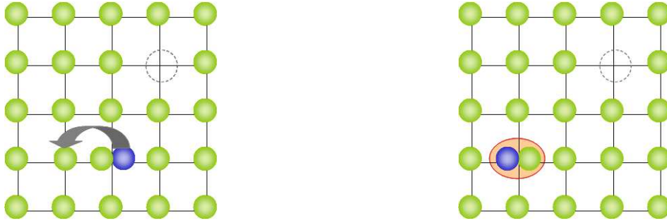
Figure 5.14: Left panel: Normal state with one mobile down-atom and one mobile up-hole. Right panel: Superfluid state with a bound molecule and one mobile up-hole.
