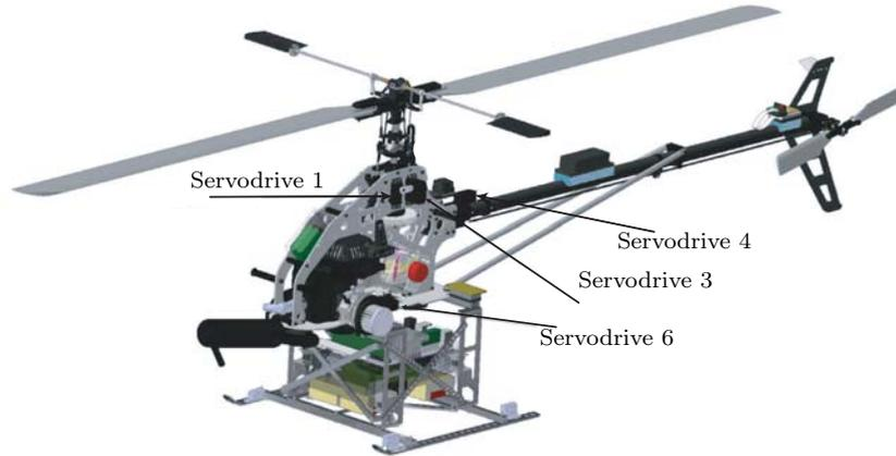
FIGURE 4.4. Three dimensional view of the CATIA® model (©Dassault Systèmes) of our helicopter. 680 different parts are modeled and kinematically linked together. Payload, landing-gear, sensors, electronic devices, Li-Po batteries, and numerous add-ons are modeled to obtain accurate estimates of inertia matrix and position of the center of gravity.
