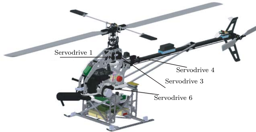
FIGURE 4.4. Three dimensional view of the CATIA® model (©Dassault Systèmes) of our helicopter. 680 different parts are modeled and kinematically linked together. Payload, landing-gear, sensors, electronic devices, Li-Po batteries, and numerous add-ons are modeled to obtain accurate estimates of inertia matrix and position of the center of gravity.
