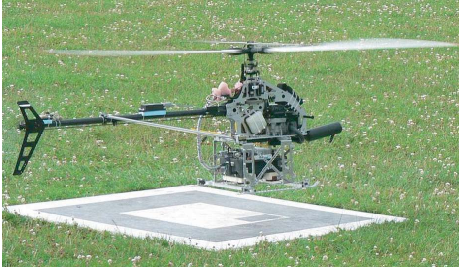
FIGURE 4.1. “Goliath”, our helicopter equipped with low-cost sensors in hover flight.
