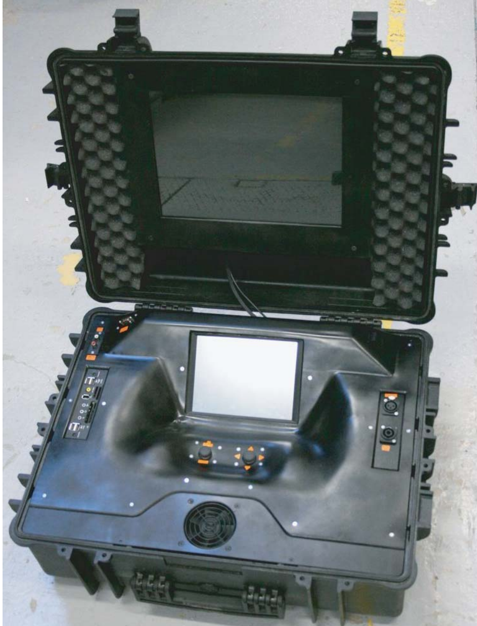
FIGURE 4.6. The latest version of our ground station fits inside a single suitcase loaded with batteries for outdoor experiments.
