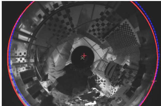
Figure 3.1: Extraction of the mirror border for the estimation of the principal point
