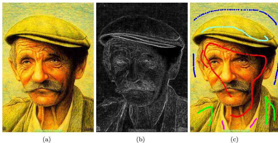
Figure 5.11: Watershed Segmentation based on local dissimilarity for color images. (a) Original color image (389x550). (b) Color gradient. (c) Markers.
