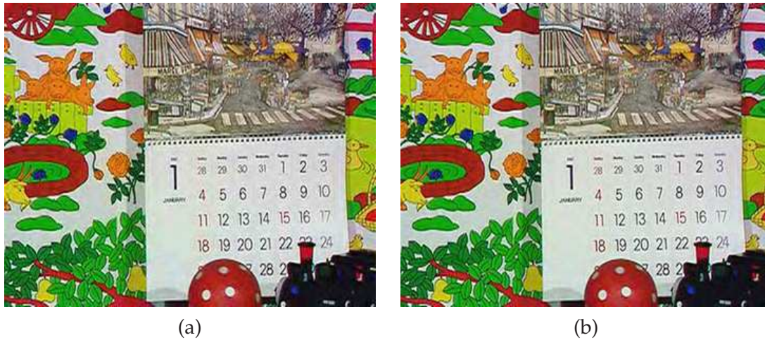
Figure 4.7: Reconstructed frame from Mobile (CIF, 30Hz) sequence at 384 kbs: (a) 5-level 9/7 spatial decomposition, (b) 5-level joint 9/7 spatial decomposition at GOP level.
