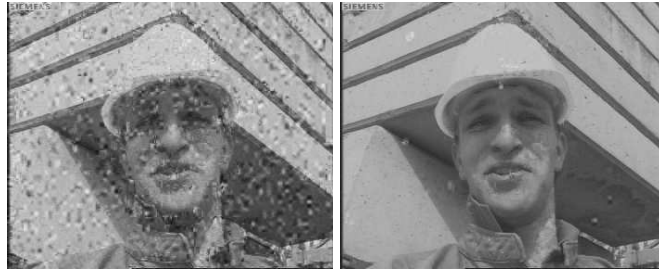
Figure A.3: Reconstructed frames after transmission on a flat Rayleigh fading channel, both with (right) and without (left) a rotation matrix. Channel SNR is 8.0 dB.
