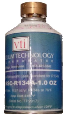
Figure 2.7 HFC-134a calibrated leak.
