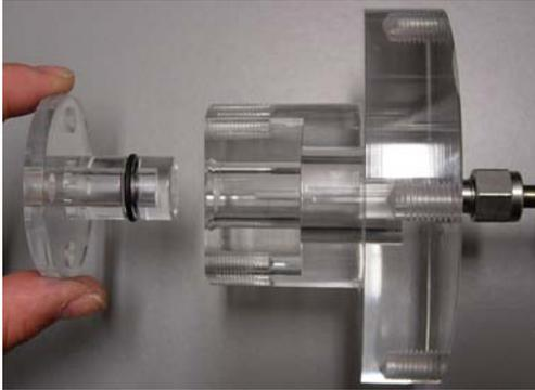
Figure 4.24 Transparent fitting specimen.
