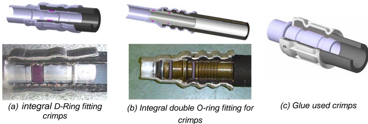
Figure 1.9 Different types of crimps (by courtesy of MAFLOW).
