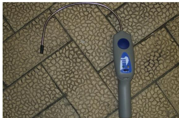
Figure 2.27 Leak detector.
