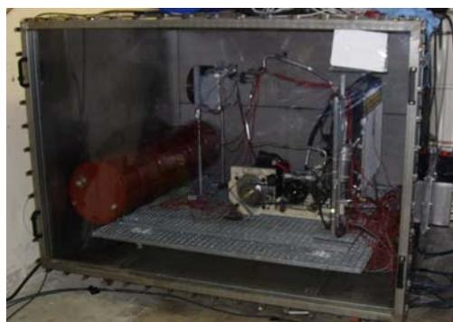
**Fig. 19. Test bench for leak flow rate test in running mode of MAC system.**
