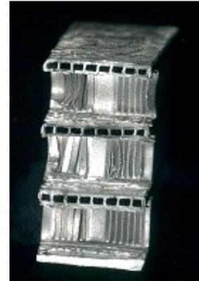
Figure 1.11 Condenser and the micro-channel structure
