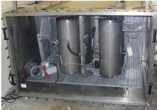
Fig. 11. Test chamber used for LFR tests of MAC system.
