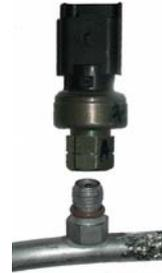
Figure 1.16 High-pressure sensor.
