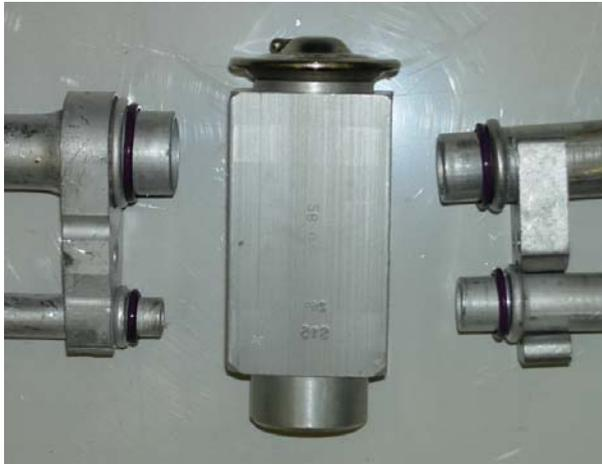
Figure 1.13 Photo of "H block" type TXV.
