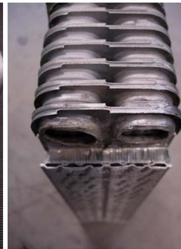
Figure 1.12 Evaporator and the micro-channel structure
