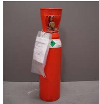
Fig. 4. Standardized gas of HFC-134a/N<sub>2</sub>.
