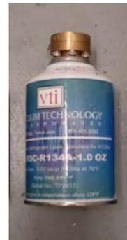
Fig. 5. HFC-134a calibrated leak.
