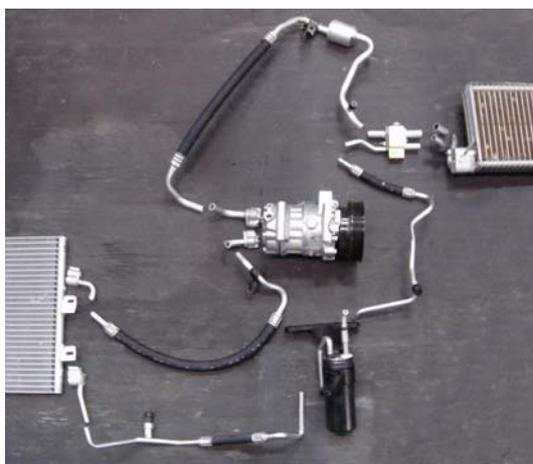
Fig. 14. MAC system cut into parts making macro-components.
