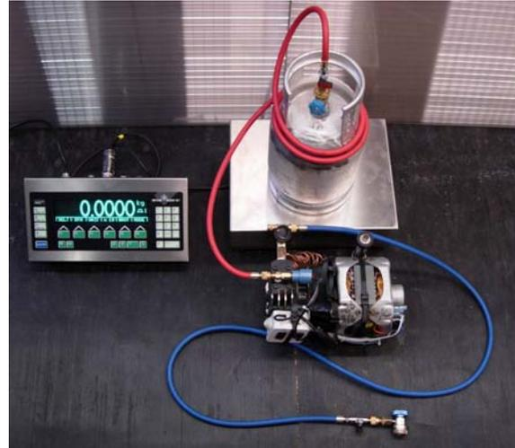
Figure 2.37 Refrigerant Recovery equipment.
