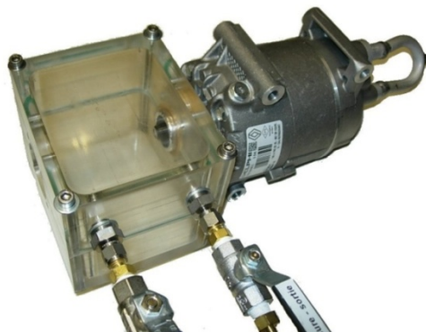
Figure 2-46 Photo of the accumulation volume to leak test the shaft seal in standstill mode.
