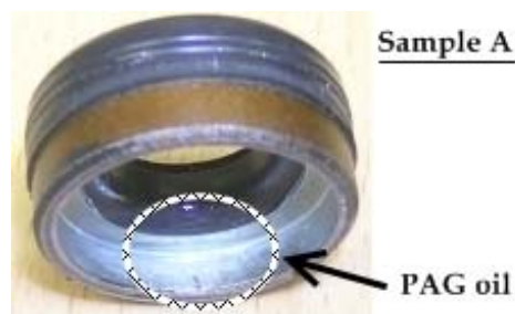
Figure 3-26 Lubricated oil at the seal low-pressure side resulting from its transportation through the seal contact.
