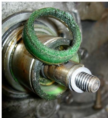
Figure 2-54 Felt ring of aged compressor C1 showing high oil leakage.
