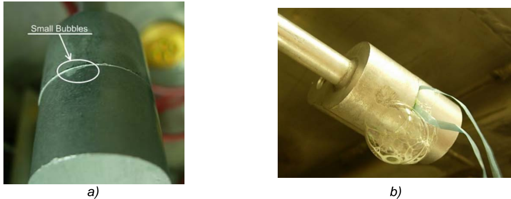
Figure 1-17 Bubbles formation for an overall leak of; a) 120 g/yr; b) 1,200 g/yr.
