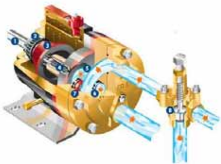
Figure 3.20 – Diaphragm pump principal of operation [HYDRACELL].
