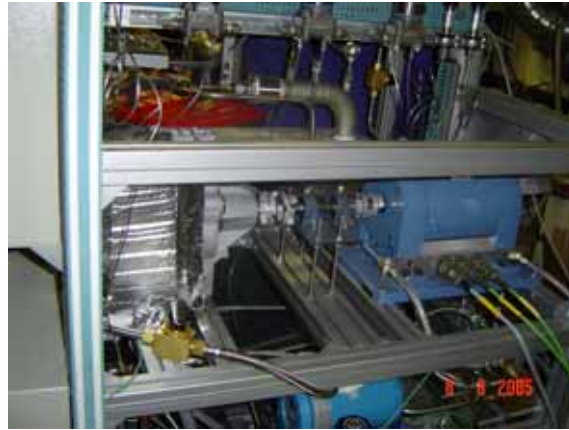
Figure 3.42 – Turbine and eddy current brake coupling.
