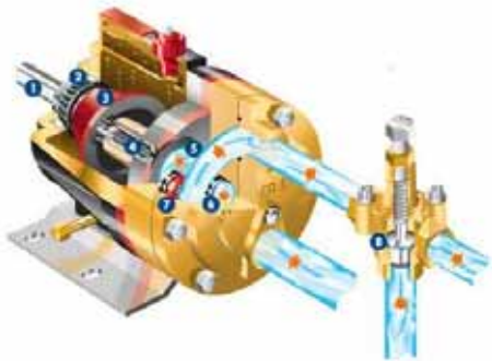
Figure 3.20 – Diaphragm pump principal of operation [HYDRACELL].
