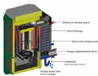
Figure 3.5 – Condensing pellet-heating system. [Okefen]
