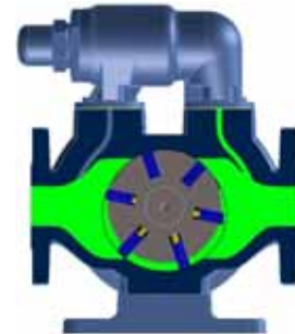
Figure 3.19 – Vane pump layout [VIKINGPUMP].
