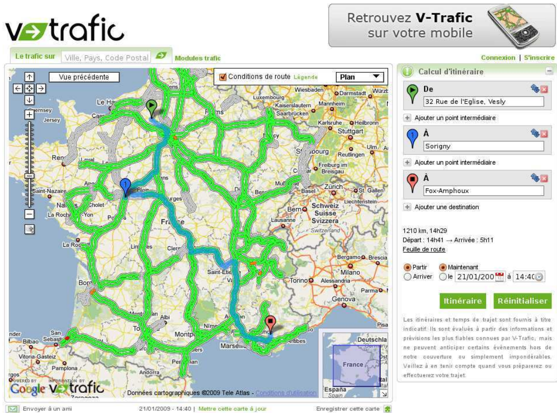
Figure 6.1: The Mediamobile web site with the route planning module. The screenshot has been taken on the beta version of the web site, which employs the TDCALT algorithm through the platform discussed in this section.
