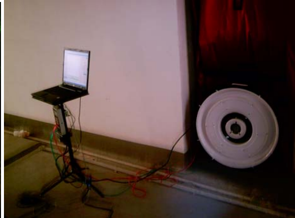
Figure 8-3 air tightness check
