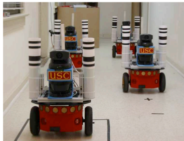
Figure 6.1: Example of tagged robots used in collaborative indoor mapping. From [221]
