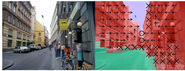
Figure 4.13: Example of machine learning based ground detection. From [188]
