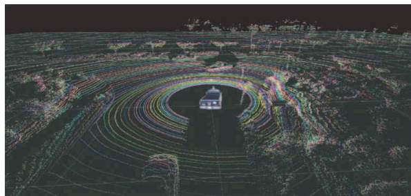
Figure 3.4: Velodyne high definition 360° lidar output. From [58]
