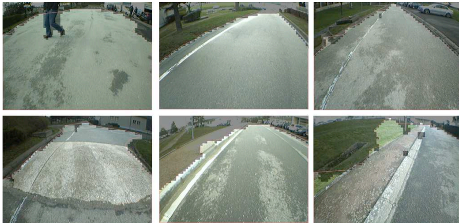
Figure 4.17: Examples of the machine learning method results. The last two images on the bottom-right show some of the failure modes
