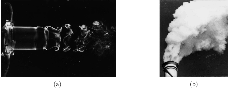
Figure 2.6: Example of jet flows. (a) KH instability in an axisymmetric jet. (b) Turbulent jet out of an industrial chimney.
