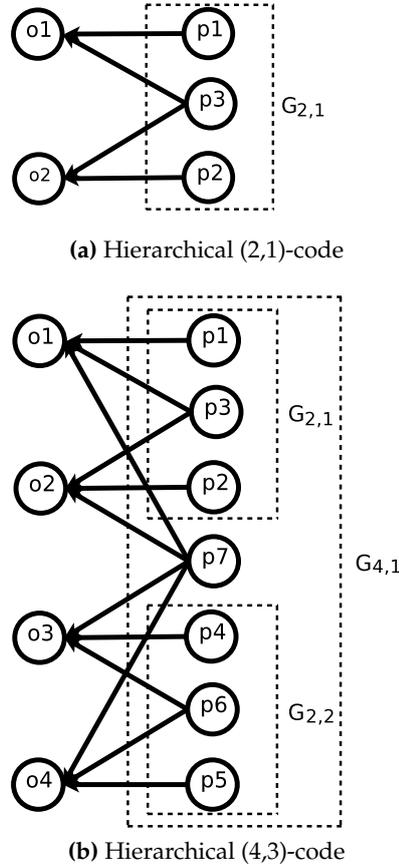
Figure 5.4: Samples of Code Graphs for Hierarchical Codes.
