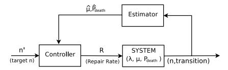
**Figure 6.1:** The adaptive control scheme.
