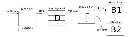
**Figure 1.6:** Data layout in CFS.
