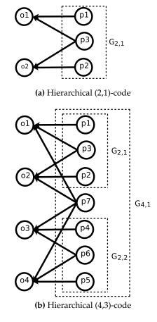
**Figure 5.4:** Samples of Code Graphs for Hierarchical Codes.
