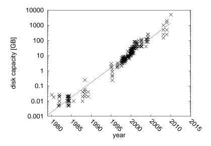
**Figure 1.2:** Capacity of hard disk over the time.
