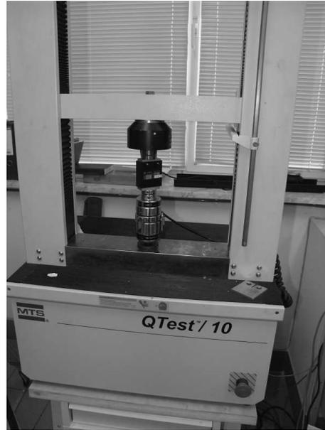
Figure F.7: Electromechanical testing stand for compression tests on CEL2-based biomaterial samples
