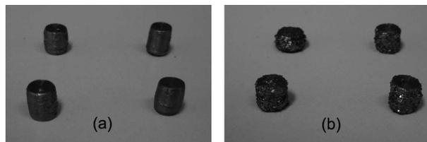
Figure E.5: Photographs of tested samples: (a) dense titanium; (b) porous titanium
