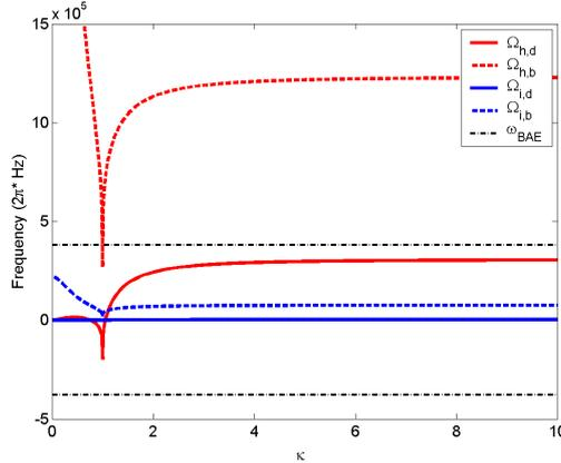
Figure 5.1: Equilibrium characteristic frequencies, calculated assuming  $R_0 = 2.45\text{m}$ ,  $q = 1$ ,  $s = 0.1$ ,  $r = 0.14\text{m}$ , 400keV hot hydrogen ions, and 3keV thermal ions. Those quantities are given as function of the pitch angle  $\kappa^2 = 2(r/R)\lambda / (1 - (1 - r/R)\lambda)$ , such that  $\kappa > 1$  corresponds to trapped particles, and  $\kappa < 1$  to passing particles.
