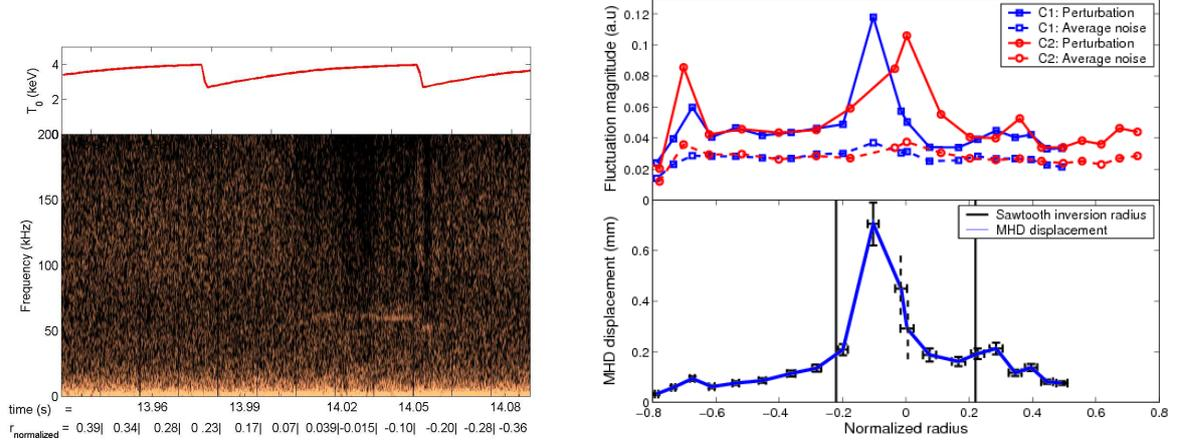
Figure 4.4: In the left hand side figure, the time spectrum of density oscillations has been plotted, for the different radii successively targetted by the reflectometer.  $-/+$  are used to distinguish high field side radii from low field side radii.
