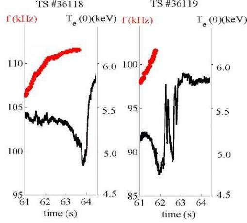
Figure 2.5: Frequency spectrum of Reversed Shear Alfvén Eigenmodes (RSAEs) identified in Tore-Supra [32]. Frequency cascading is associated to both density fluctuations and oscillations of the  $q$ -profile.
