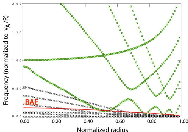
Figure 4.1: Continuum spectrum calculated with CSCAS [86], based on the CRONOS transport reconstructed equilibrium for shot #42039 ( $t \sim 9.5$ s), whose main characteristics can be found in Figs. 5.4 and 5.5. The spectrum is plotted for a mode with a toroidal mode number  $n = 1$  and an assumed compressibility of 1.67. The green curves correspond to the lines of the Alfvén spectrum, the black curves to the slow continuum.
