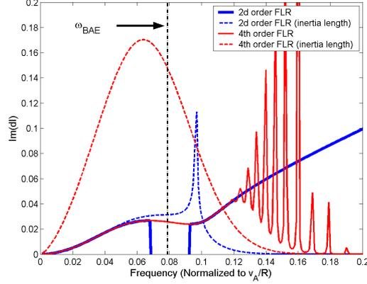
Figure 5.2: Inertia localized damping,  $\text{Im}(\delta\hat{I})$ , as a function of the real frequency  $\omega_r$  for the different models given by formulas 5.12 and 5.16. Below  $\text{Re}(\Lambda^2) = 0$  represented by the divergence of the blue dotted curve, damping is to be attributed to Landau damping, whereas continuum damping dominates for  $\text{Re}(\Lambda^2) > 0$ .
