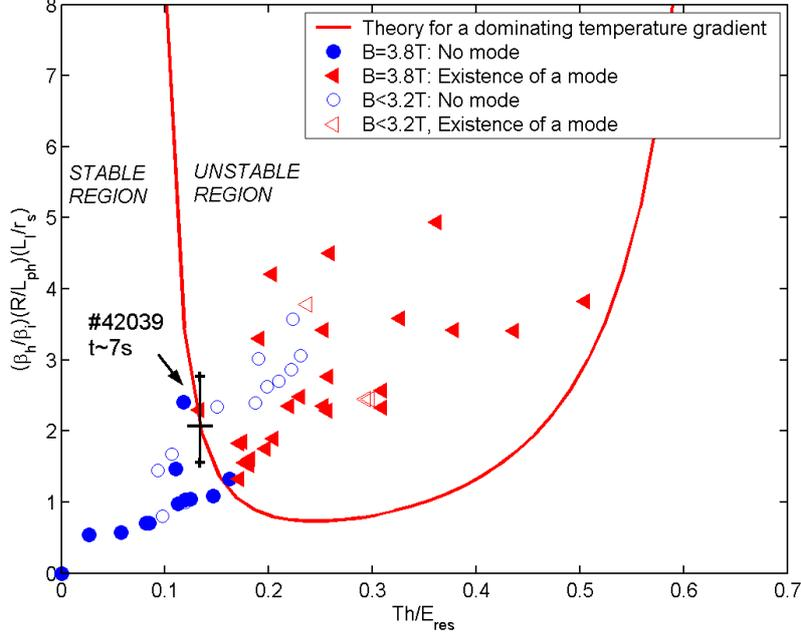
Figure 5.9: BAE apparitions in Tore-Supra discharges, compared to the theoretical prediction. A “mode observation” corresponds to a coherent signal/noise value exceeding 2. The pointed dot corresponds to the case #42039,  $t \sim 7s$ .
