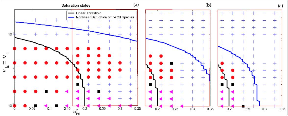
Figure 6.7: Stability diagrams corresponding to  $m_d/m_l = 0.5$ ,  $\nu_d = 0.005$ , for various magnitudes of the initial perturbation:  $\omega_{Bb}(t = 0) = 0.1$  in Fig. (a),  $\omega_{Bb}(t = 0) = 0.05$  in Fig. (b),  $\omega_{Bb}(t = 0) = 0.025$  in Fig. (c).
