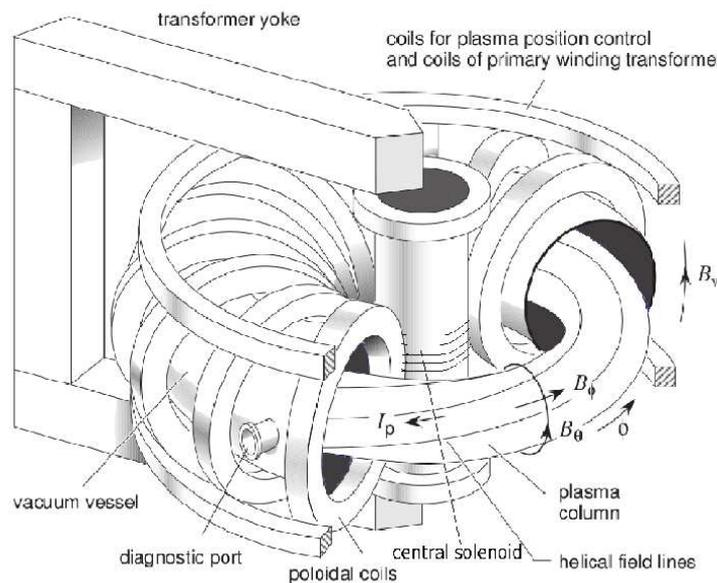
Figure 1.3: The tokamak and its confining magnetic set-up.
