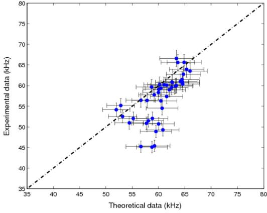
Figure 4.5: Comparison of  $\omega_{BAE}$  with the experimental frequencies (averaged over 10ms windows, to avoid the details of the mode frequency evolution faster than the temperature relaxation time) between 40kHz and 80kHz and exceeding a signal/noise value of 3., for the full set of our experiments with  $P_{LH} = 0$ . Horizontal errorbars correspond to an assumed 30% error on the value of  $T_e/T_i$ .
