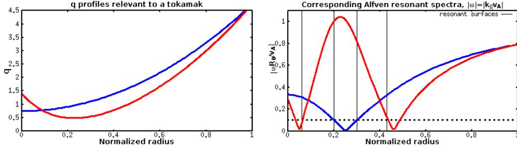
Figure 2.3: Typical sheared  $q$  profiles of a tokamak and corresponding Alfvén resonant spectra for modes with a single poloidal and toroidal component, ( $m = -1, n = 1$ ). As an example, the resonant surfaces for an acoustic mode ( $\omega R_0/v_A \sim \beta \sim 0.01$ ) are indicated, and show where such a mode should display a singularity.
