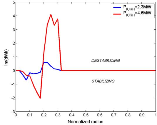
Figure 5.8: Radial profile of the fast ion induced wave-particle energy transfer,  $\text{Im}(d\hat{W}_k(\bar{r}))$ , for different power input.  $\text{Im}(d\hat{W}_k(\bar{r}))$  verifies  $\int_{\bar{r}} d\bar{r} \text{Im}(d\hat{W}_k(\bar{r})) = \text{Im}(d\hat{W}_k)$  with  $\bar{r}$  the normalized radius.
