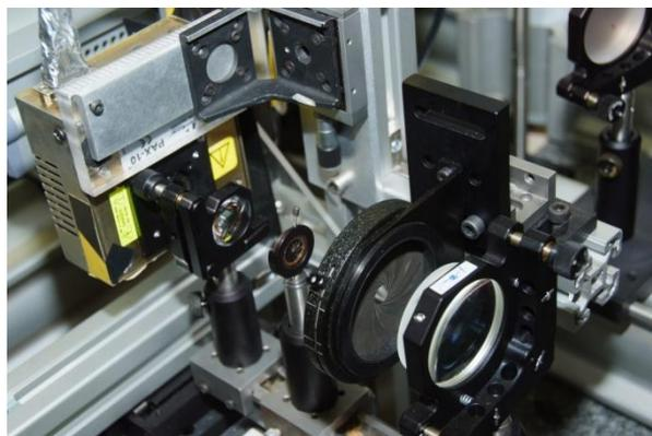
fig 3.30 picture of the Perkin xenon flashlamp and the parallel beam output.
