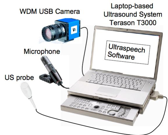
Figure 1: Hardware component of the acquisition system
