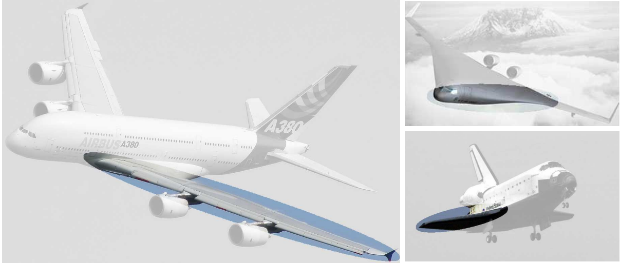
Figure 1.1. Typical examples of compressible flow about a yawed blunt body: subsonic flow about the swept wings of a civil aircraft (left), swept leading-edge flow about a blended wing-body (BWB) aircraft, a concept for future aircraft (top right), and hypersonic flow about the swept wings of a space shuttle (bottom right).
