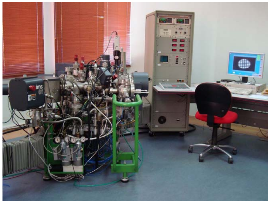
Figure 3.10: Cameca ims 6f secondary ion mass spectrometer used in this study.
