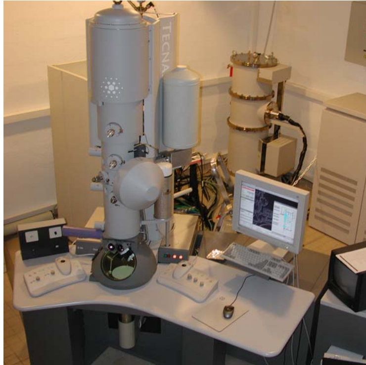
Figure 3.7: TECNAI F 20 ST TEM used in the study.
