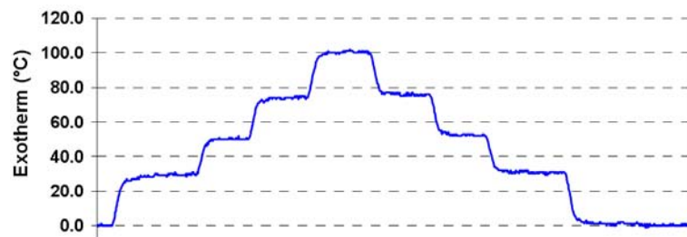
Figure 7.3: Illustration of a typical T^{out} - T^{in} profile caused by control HC u step increases and decreases. T^{in} remains roughly constant during the test.
