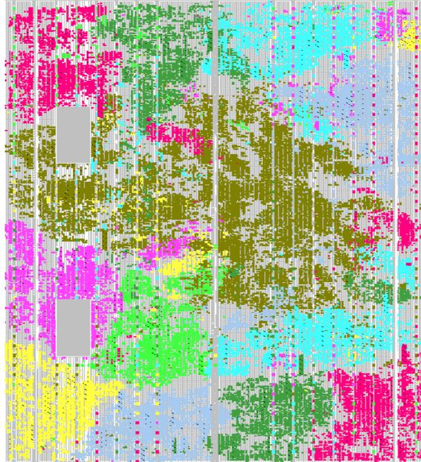
**Figure 6.7 Multiprocessor Xilinx FX140 floorplan (un-optimized)**
