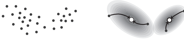
Figure 8.13: Mean-shift clustering. Given a set of samples \{u^i \in \mathbb{R}^d\}_{i=1}^N (left), the mean-shift algorithm proceeds as a hill-climbing procedure on the estimated density \hat{f}_h (right). Each sample u^i is moved iteratively towards a local maximum of the density (white circles). Final clustering is given by the assignment of the original samples to the detected maxima.
