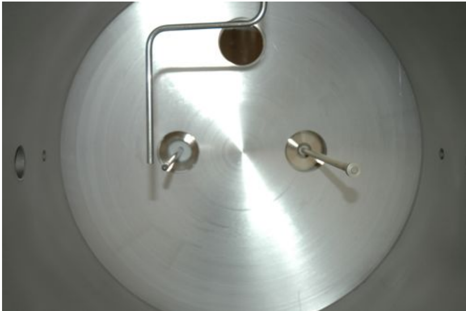
Figure 3.8: Filament probe (left) and planar probe (right) installed on the end panel of the thruster chamber.
