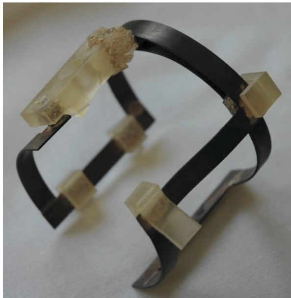
Figure 4.1: Boswell-type (double-saddle) antenna used in the first design of the PEGASES thruster prototype I, after it was removed from the thruster.
