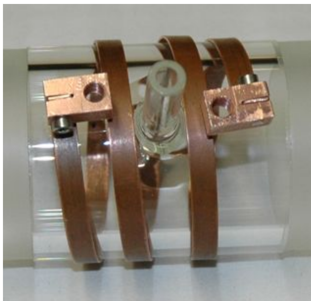
Figure 4.2: Three-coil antenna wrapped around the thruster cylinder and centered around the gas injection.
