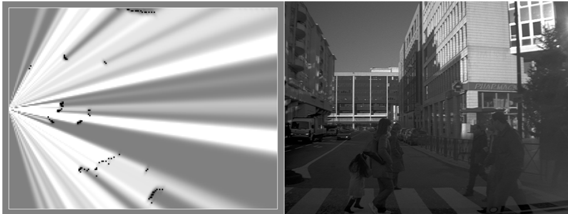
Figure 2.15: Example of an occupancy map representation. White cells are free and black ones occupied.
