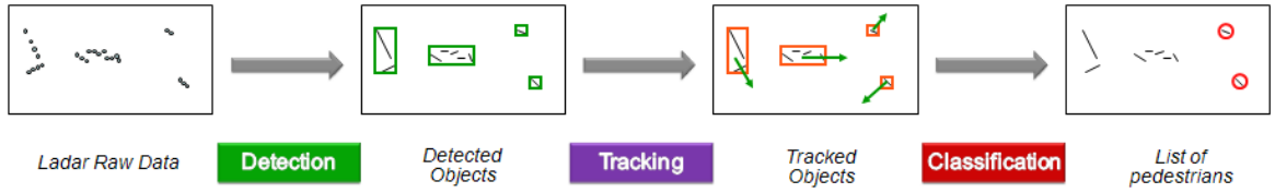
Figure 3.7: Schematic view of the ladar sub-system data flow.
