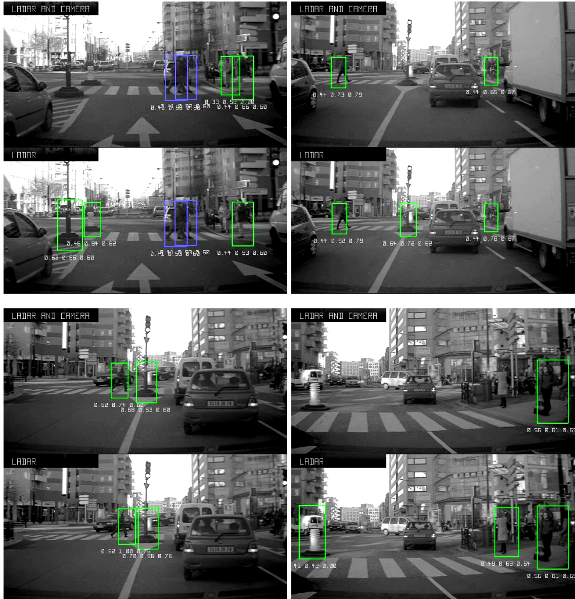
Figure 3.33: Example of the proposed complete system output in real situations. The corresponding output of the ladar sub-system is also given for comparison below each snapshot. Obstacles detected as groups are shown as blue rectangles (the basic routine mentioned in section 3.5.2 is used here to discriminate roughly pedestrians inside "groups"). The three numbers visible below each rectangles are the three uncertainty scores mentioned in this chapter. The two last figures show situations where the system fails to compute the correct list of pedestrians present in the scene.
