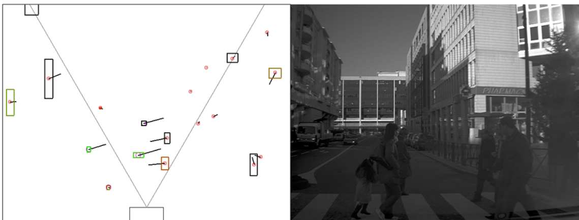
Figure 2.14: Example of a features based representation where the position, velocity vector and dimension of the outlining box is estimated for each object in the environment.
