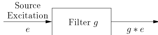
Figure 3.4: Source/Filter model: the glottal source excitation e is filtered by filter g , leading in the time domain to the convolution g * e .
