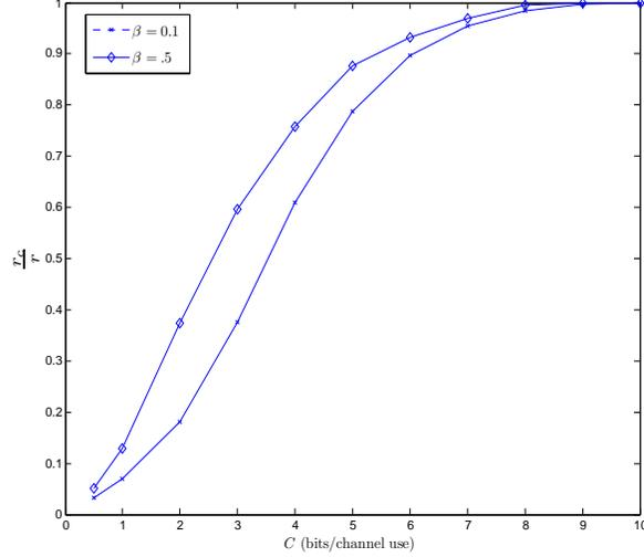
Figure 6.3: Average common to total rate Ratios vs. Backhaul capacity for Max Min Rates,  $N_t = 1$ , SNR = 10dB,  $\mathbf{h}_{k,k} \sim \mathcal{CN}(0, \mathbf{I}_{N_t})$  and  $\mathbf{h}_{k,\bar{k}} \sim \mathcal{CN}(0, \beta \mathbf{I}_{N_t})$ .
