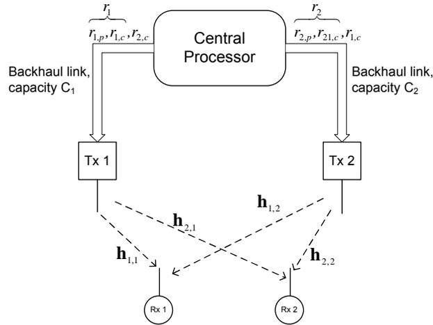
Figure 6.1: Constrained backhaul setup.
