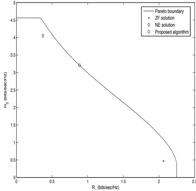
Figure 4.2: Pareto rate boundary, MRT, ZF and  $\alpha_{12} = \alpha_{21} = 1$  points for a channel instance sampled from a channel with i.i.d.  $\mathcal{CN}(0, 1)$  coefficients,  $N_t = 3$ ,  $K = 2$ .
