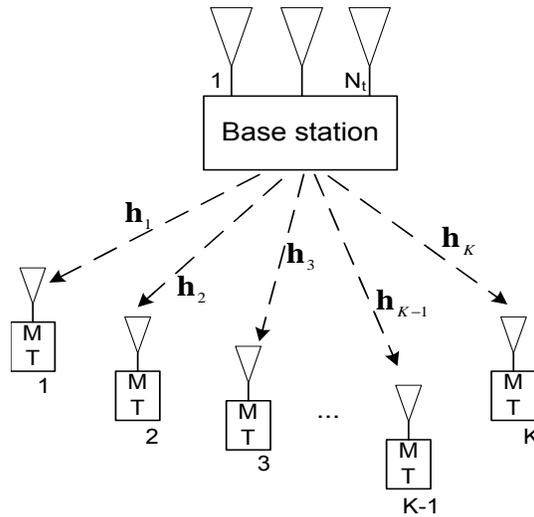
Figure 2.2: MIMO Broadcast Channel, Single Cell Setup with  $N_t$  antennas at the transmitter and  $K$  single antenna receivers.  $\mathbf{h}_k \in \mathbb{C}^{1 \times N_t}$  denotes the channel coefficients vector of the DL channel from the base station to user  $k$ ,  $k = 1, \dots, K$ .
