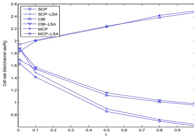
Figure 7.6: Comparison between average normalized cell rates achieved by the optimization problems in Section 7.3 and the large system analysis results for  $K = 3$ ,  $N_t = 4$  and  $\text{SNR} = 10\text{ dB}$ .
