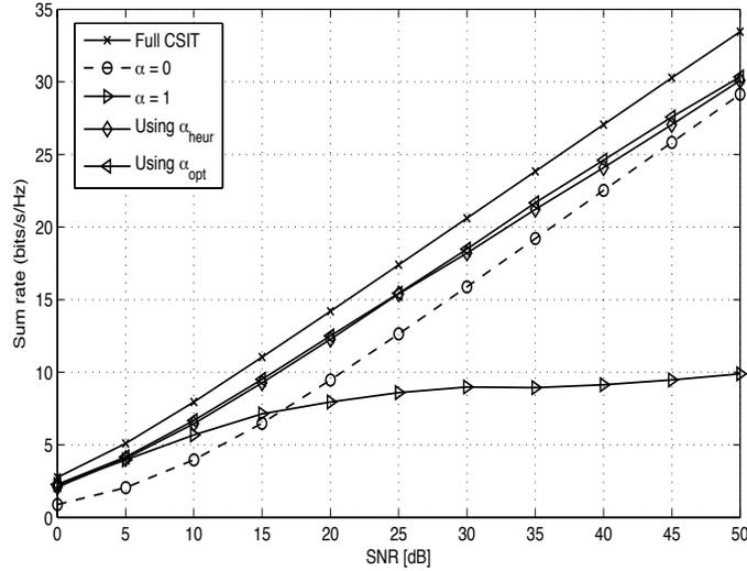
Figure 3.4: Average sum rates for  $N_t = 2$ ,  $K = 30$ ,  $B_{\text{total}} = 120$  bits, and different schemes.  $\alpha_{heur}$  provides a smooth transition between extreme  $\alpha$ 's, with tolerable loss with respect to  $\alpha_{opt}$ .
