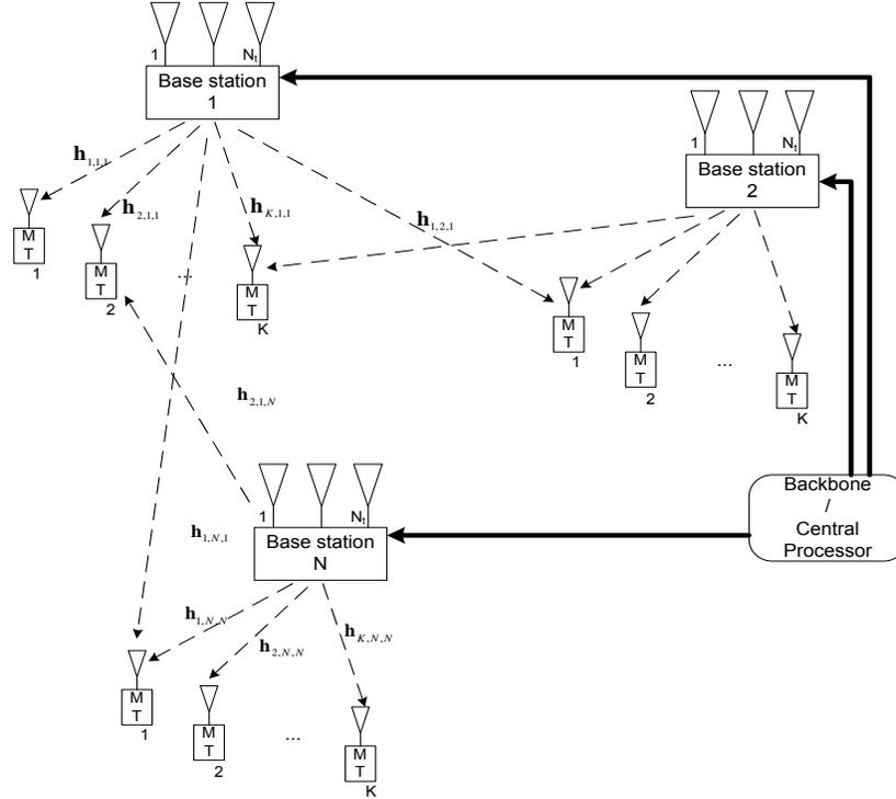
Figure 2.3: MIMO Broadcast Channel, Multicell Setup with  $N_t$  antennas at each base station and  $K$  single antenna receivers in each cell.  $\mathbf{h}_{k,j,\bar{j}} \in \mathbb{C}^{1 \times N_t}$  denotes the channel coefficients vector of the DL channel from base station  $\bar{j}$  to user  $k$  in cell  $j$ ,  $k = 1, \dots, K$ ,  $j, \bar{j} = 1, \dots, N$ .
