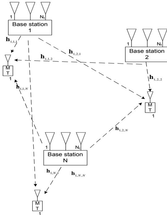
Figure 2.4: MISO IC, Multicell Setup with  $N_t$  antennas at each BS and  $K$  single antenna receivers in each cell.  $\mathbf{h}_{k,j,\bar{j}} \in \mathbb{C}^{1 \times N_t}$  denotes the channel coefficients vector of the DL channel from BS  $\bar{j}$  to user  $k$  in cell  $j$ ,  $k = 1, \dots, K$ ,  $j, \bar{j} = 1, \dots, N$ .
