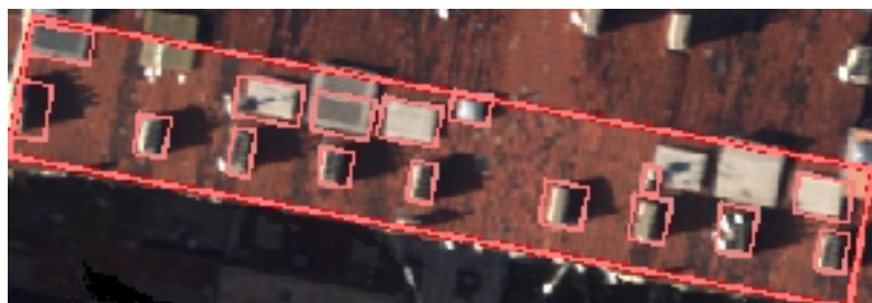
Figure B.4: The detected and reconstructed superstructures using the exhaustive search-based method (Chapter 3).
