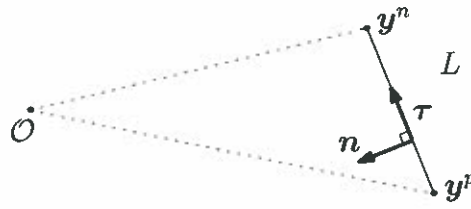
FIGURE 5.5. Geometry of segment L , unit tangent vector \tau and unit normal vector n .
