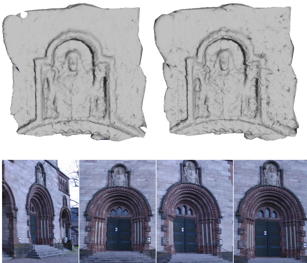
Figure 5.5: Mesh obtained by the method of [Pons et al., 2007] initialized by the output of: a) our method b) The multi-view reconstruction method [Labatut et al., 2007]. c) Some images of the Herz-Jesu-P8 dataset. We have used only a partial cut of the original images.
