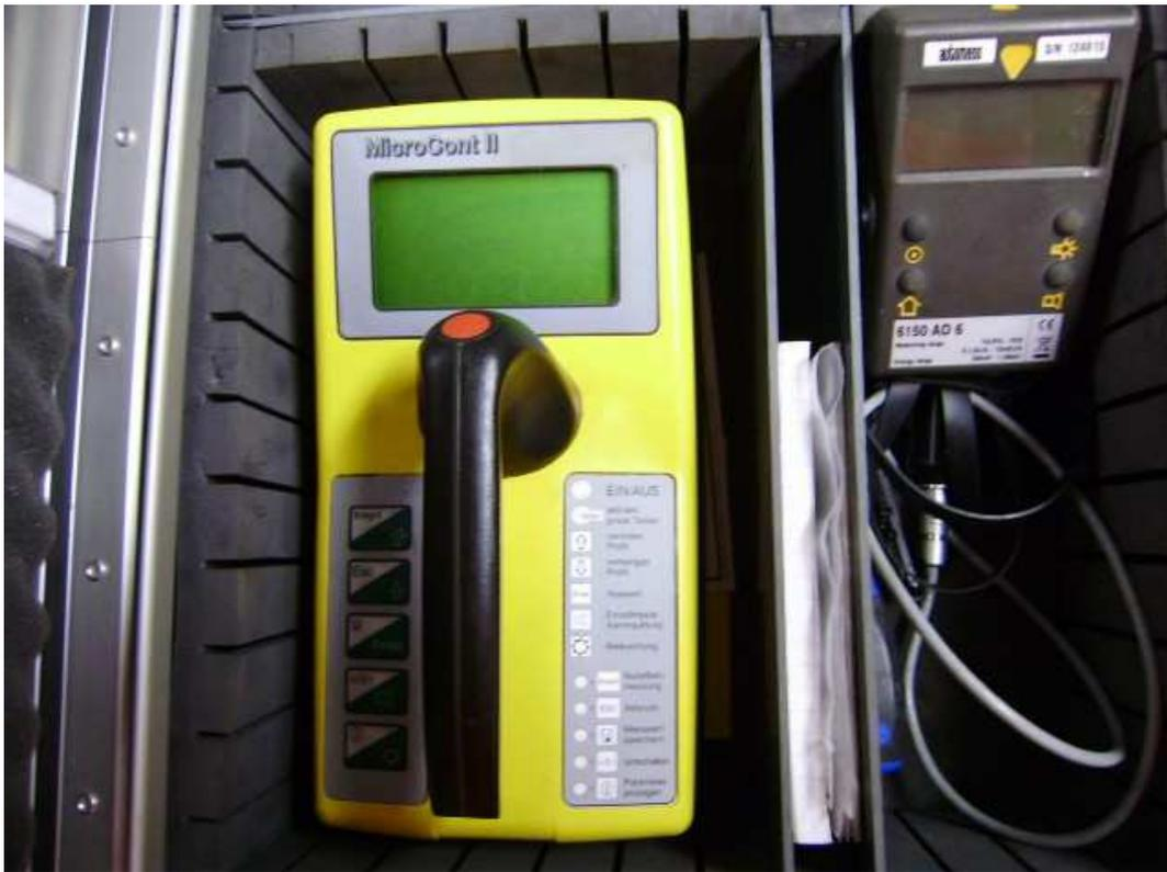
*Illustration 10: A hand-held radiation gauge of the type used offshore.*
