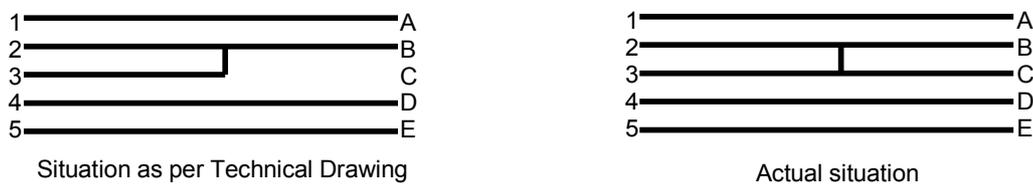
*Illustration 20: Simplified diagram illustrating the difference between Technical Drawing and actual situation. Note connections 2-B and 3-C.*
