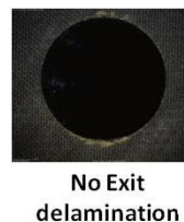
Figure 7. Performance of Reference D in Ti6Al4V-CFRP stacks
