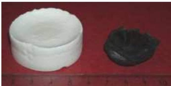
**Figure IV-8:** Cellulose-containing OA PC (left) and its carbonaceous counterpart CA PCC (right)
