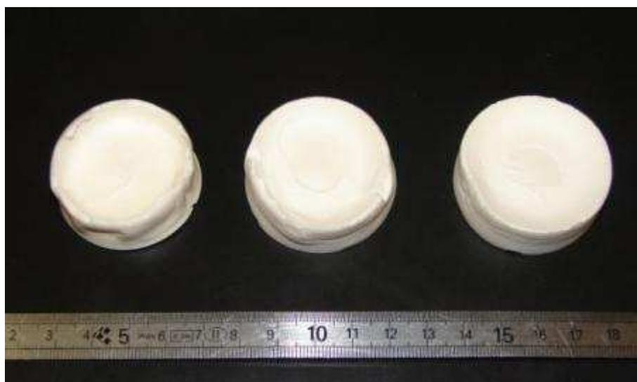
**Figure IV-7:** Cellulose-containing aerogels PA containing 5 %Cellulose (left), PB containing 10 %Cellulose (middle), and PC containing 15 %Cellulose (right)
