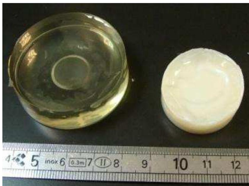
**Figure II-14:** Cellulose-acetate based gel and aerogel (after drying in supercritical CO<sub>2</sub>) 10-0.2-0.25DA
