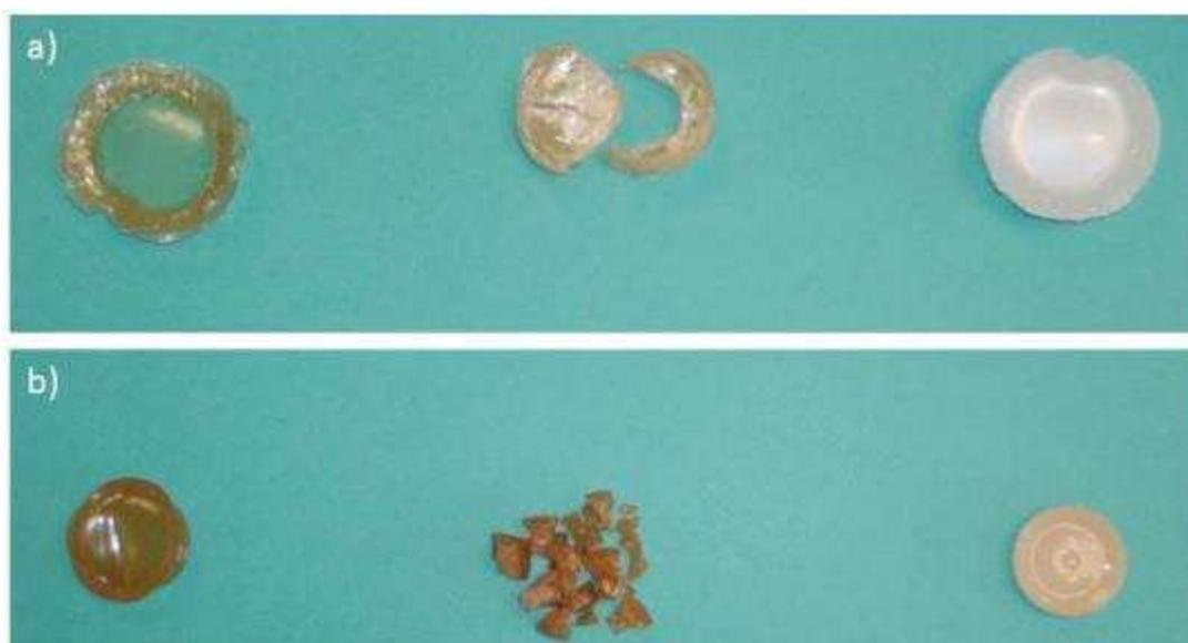
**Figure II-26:** Comparison of the effects of drying by evaporation in air (left), lyophilisation (middle), and supercritical drying in CO<sub>2</sub> (right) on samples a) 10-0.1-8DD and b) 5-1-1DD
