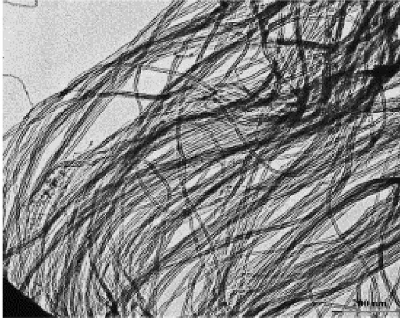
**Figure I-9:** TEM images of carbon nanotubes obtained over Fe,Co/zeolite catalyst aligned into bundle-like structure [Her 2004]
