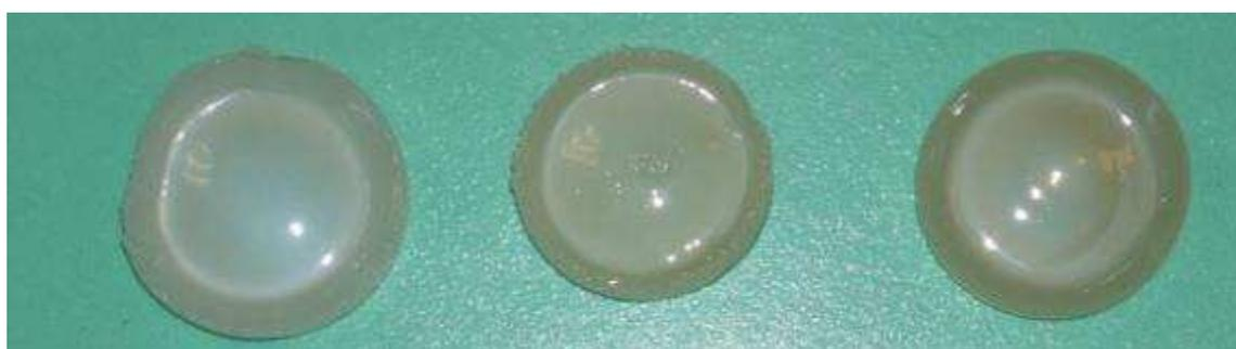
**Figure II-17:** CAB aerogels having been synthesized using different catalysts: 15-0.1-5DD (left), 15-0.1-1DA (middle), 15-0.1-25P (right)
