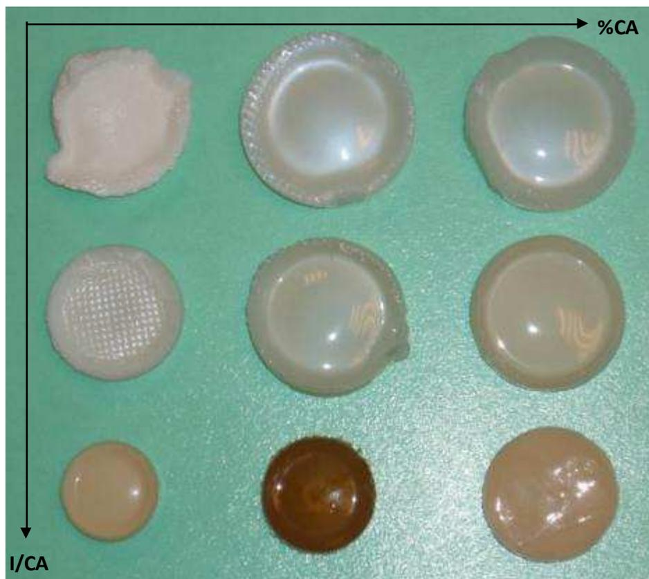
**Figure II-16:** CAB aerogels having been synthesized %CA and I/CA: 3-0.1-5DD, 10-0.1-5DD, 15-0.1-5DD, 3-0.2-5DD, 10-0.2-5DD, 15-0.2-5DD, 3-1-5DD, 10-1-5DD, 15-1-5DD (from left to right and top to bottom)
