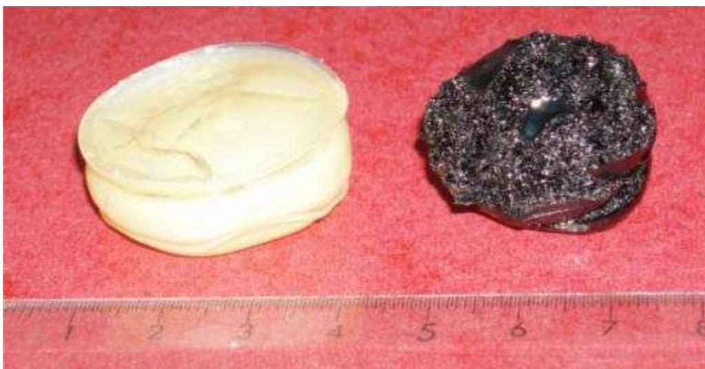
*Figure III-2: Aerogel 15-0.2-100P before and after pyrolysis at 1000°C in  $N_2$*
