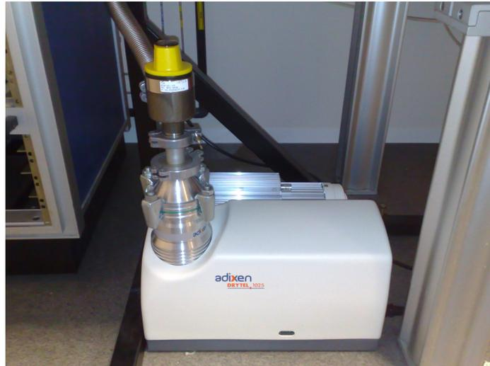
**Fig. 3.18:** The Adixen turbo pump used for creating the vacuum into the chamber for the test, figure 3.19. This setup allowed us to place and control the device into the chamber..
