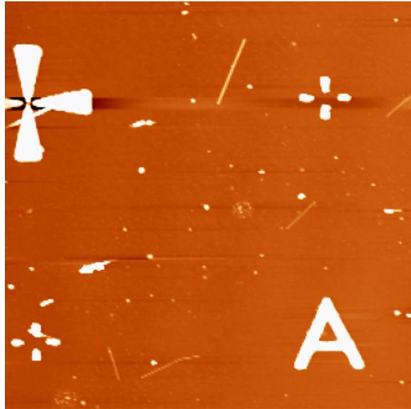
**Fig. 5.3:** Localisation of CNT-s through AFM imaging
