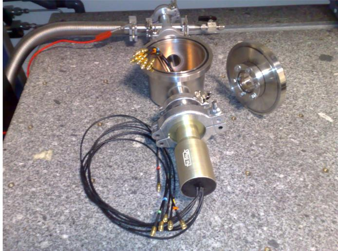
**Fig. 3.16:** The vacuum chamber setup used for low pressure measurements
