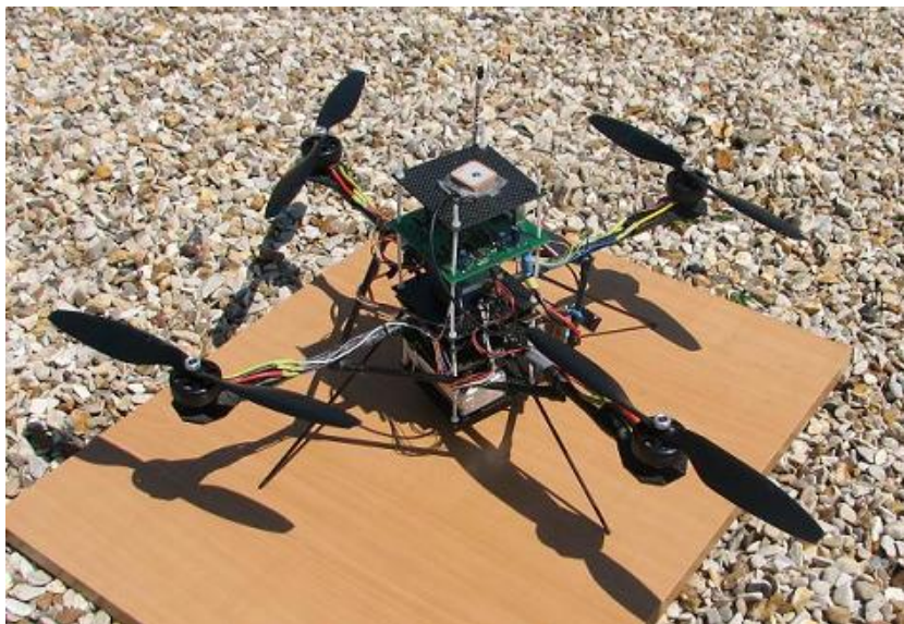
FIGURE 6.1. Our home-built quadrotor: the “Quadricopter”.
