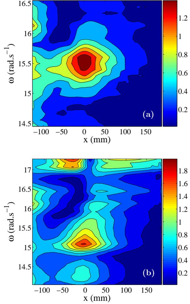
Fig. 3: Evidence of the trapped mode resonances:  $(h_T(x, y, t) - h_T(x, -y, t)) / 2$  for some fixed  $y$  is displayed in colorscale as a function of  $x$  and  $\omega$ . (a) for  $a/d = 0.50$ , one resonance is visible near the cylinder and (b) for  $a/d = 0.85$ , in addition to the first resonance, a second maximum near the cutoff frequency can be seen (the cylinder lies at  $x = 0$ ). The scale of the colorbar is in mm.
