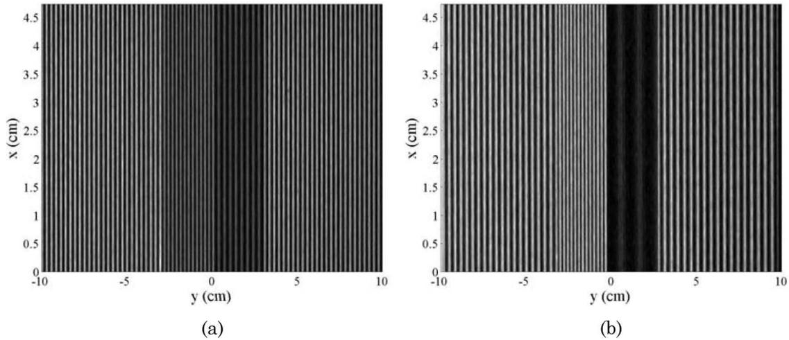
Fig. 6. Experimental intensity variations  $I(x,y)$  captured by the camera (a) in the parallel-optical-axes geometry with  $D = 18$  cm and  $L = 105.2$  cm and (b) in the crossed-optical-axes geometry with  $D = 70.7$  cm ( $\theta = 33.9^\circ$ ),  $L = 105.2$  cm, and  $y_0 = 0$ .
