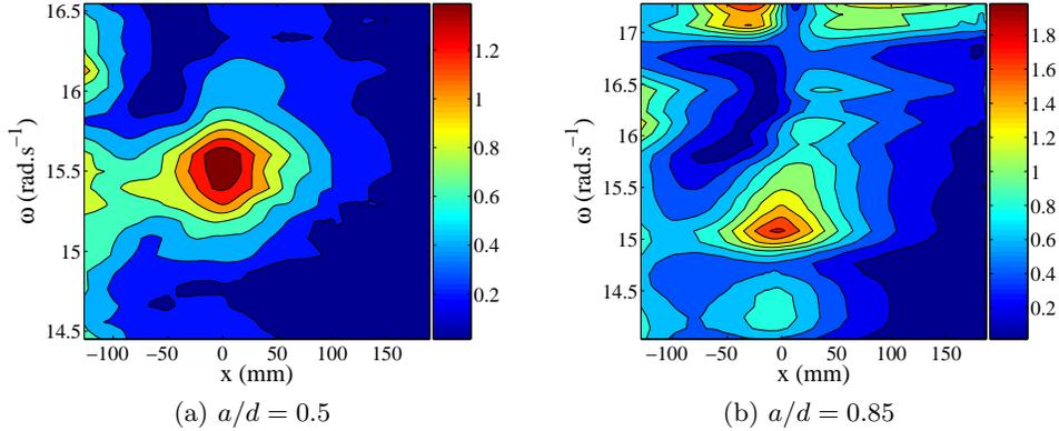
Figure 5: Experimental evidence of the trapped mode resonance:  $1/2 \cdot [h_T(x, y, t) - h_T(x, -y, t)]$  for some fixed  $(y, t)$  is displayed in color scale as a function of  $x$  and  $\omega$ . (a) For  $a/d = 0.5$ , one resonance is visible near the cylinder, (b) for  $a/d = 0.85$  in addition to the first resonance a second maximum near the cut-off frequency can be seen. The cylinder lays at  $x = 0$  mm (configuration I). The scale of the color bar is in mm.
