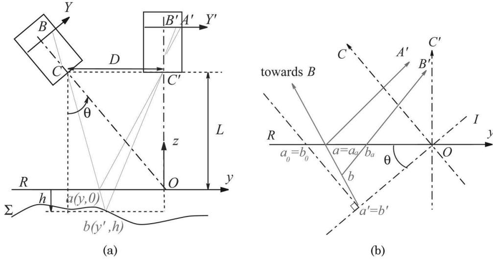
Fig. 12. (a) Reproduction of Takeda's representation and (b) the same representation including useful additional points:  $b'$  is the point of the ray  $Bb$  on the plane  $I$ ,  $b_a$  is the point of ray  $Bb'$  on the plane  $R(Oy)$ , and  $b_0$  is the point on plane  $R$  with  $b_0b'$  parallel to the projector's optical axis  $CO$ . Similar construction is used to define  $a_a$ ,  $a_0$ , and  $a'$ .
