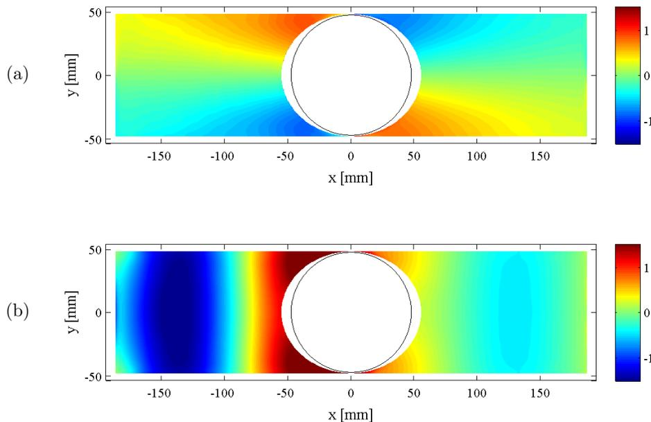
Figure 11: Experimental patterns of a second kind of trapped modes and their associated symmetric part. Panels (a-b): symmetric and antisymmetric fields of  $h_1(x, y, t)$  for  $a/d = 0.95$  and  $kd = 1.51$  ( $f = 2.62$  Hz). The position of the obstacle is indicated by the black circle. The scale of the colorbar is in mm.
