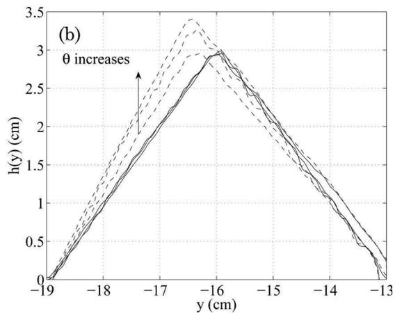
Fig. 11. Reconstructed height  $h(y)$  in the crossed-optical-axes geometry (a) for  $\theta = 33.9^\circ$  and varying the  $y_0$  position of the triangle and (b) for  $y_0 = -16$  cm and varying  $\theta = 0, 18.1$  and  $41^\circ$ . Solid curves correspond to our height reconstruction from Eq. (3.3) with Eq. (1.2). Dashed curves are the height reconstructed using Takeda's relation Eq. (1.1).
