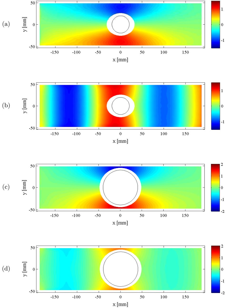
Figure 10: Experimental patterns of the trapped modes and their associated symmetric parts. Panels (a-b): Symmetric and antisymmetric fields of  $h_1(x, y, t)$  for  $a/d = 0.4$  and  $kd = 1.46$ , ( $f = 2.50$  Hz). Panels (c-d): Same representation for  $a/d = 0.80$  and  $kd = 1.33$  ( $f = 2.40$  Hz). The position of the obstacle is indicated by the black circle. The scale of the colorbar is in mm.
