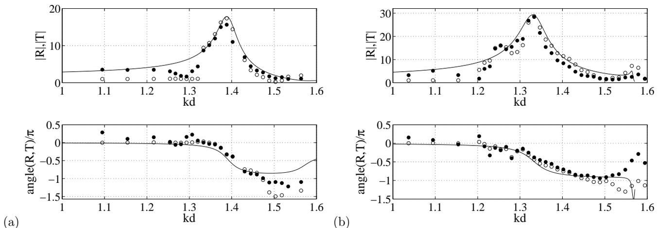
Fig. 6: Resonance curves for (a)  $a/d = 0.50$  and (b)  $a/d = 0.85$ , upper panel  $|R|$  (plain circle),  $|T|$  (open circle) as a function of the wavenumber  $kd$ . Lower panels show the corresponding phases. Plain lines correspond to the results obtained from numerical calculations, indiscernible from the expression in Eq. (4).
