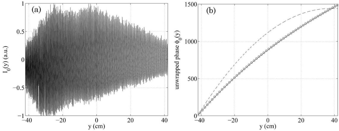
Fig. 8. (a) Intensity variations  $I_0(y)$  for fringe projection onto the reference plane in the absence of the triangular prism and (b) the corresponding unwrapped phase  $\phi_0(y)$  (see [23]). Experiments correspond to  $\theta = 33.9^\circ$  with  $L = 105.2$  cm. The points are the experimental data (only one point of each 150 points is indicated for visibility), the solid curve corresponds to our Eq. (2.12) and the dashed curve corresponds to Eq. 2.13 from [12,13,20].
