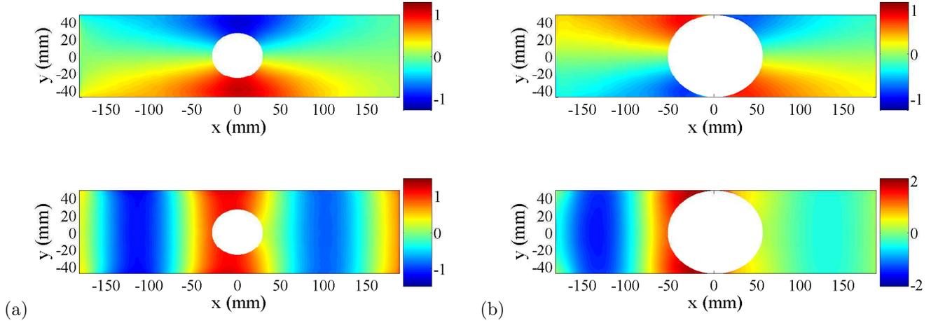
Fig. 4: Experimental patterns of the two trapped modes, and the associated even parts. (a) even and odd fields of the linear field  $h_1(x, y)$ , for  $a/d = 0.40$  and  $kd = 1.46$ . The even part exhibits the form of the trapped mode localized in the vicinity of the cylinder. (b) Same representation for  $a/d = 0.95$  and  $kd = 1.51$ . The scale of the colorbar is in mm.
