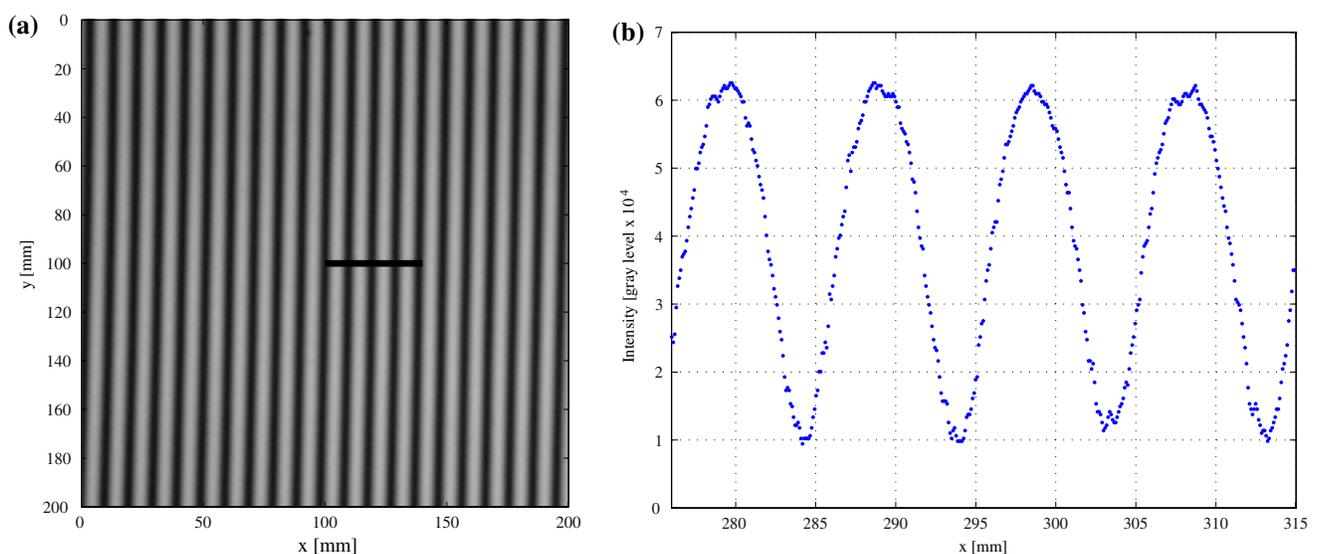
**Fig. 3** **a** Sample image of the fringes projected onto an undeformed liquid surface as registered by the camera. **b** Intensity profile along the horizontal segment shown in *black* over the image *a*
