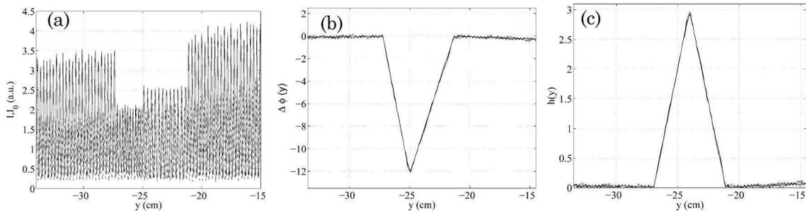
Fig. 9. (a) Signals  $I_0(y)$  and  $I(y)$  for fringe projections on the reference plane  $R$  and on the  $\Sigma$  plane. (b) Unwrapped phase difference  $\Delta\varphi(y)$  and (c) reconstructed height  $h(y)$  using Eqs. (2.9) and (2.11). The experiment is conducted in the parallel-optical-axes geometry with  $L = 105.2$  cm,  $D = 18$  cm, and  $y_0 = -24$  cm.
