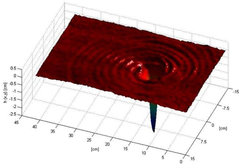
visualised spiral waves in an comparable experimental situation where they appear to be the natural solutions for a plane surface waves background flow in the presence of a vortex. An experimental study on these spiral waves is currently in progress.
