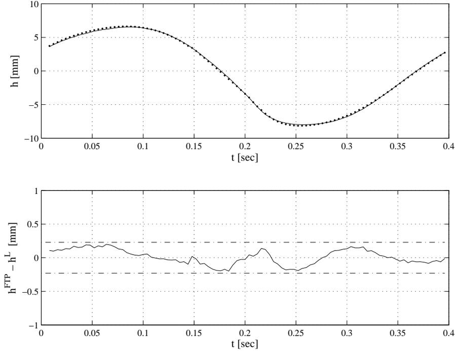
Figure 3: Comparison between two measurements made at the same point with a standard laser profilometer (plain line) and FTP at the same point (dashed line).
