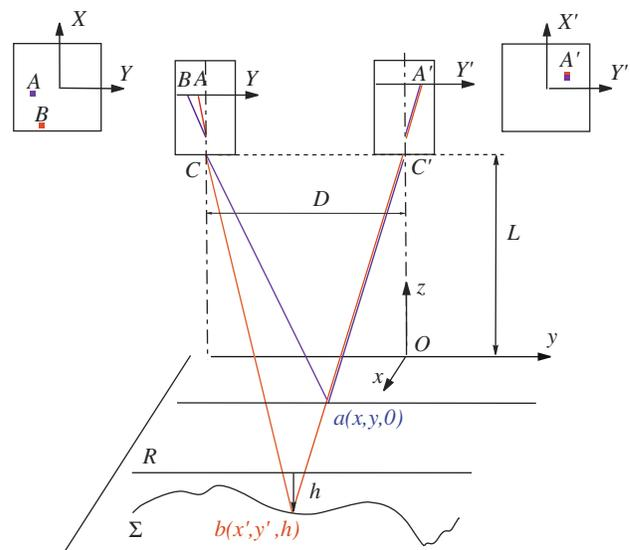
**Fig. 1** Optical configuration scheme and ray tracing for the projection and imaging system. Parallel–optical-axes geometry is adopted: both optical axes are coplanar and parallel to each other, separated by a distance  $D$ , while the entrance pupils are positioned at the same height,  $L$  over the undeformed reference surface. [The point of coordinates  $(x', y', h)$  in the figure corresponds to  $(x + \delta x, y + \delta y, h)$  in the notation used for the text]
