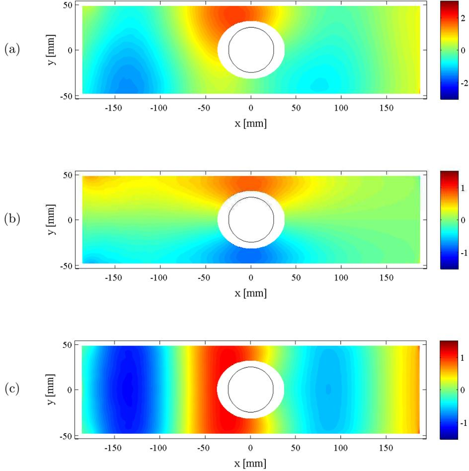
Figure 9: Linear part of the experimentally measured free-surface deformation: Type II configuration for  $a/d = 0.5$ . Panel (a) shows the linear deformation field  $H_1(x, y)$  (same as in ). Panels (b) and (c) presents the symmetric and antisymmetric parts of the linear mode  $H_1(x, y)$ , respectively. The position of the obstacle within the waveguide is indicated by the black circle. The scale of the colorbar is in mm.
