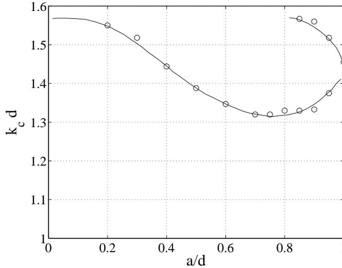
Figure 18: Variation of the trapped mode frequency parameter  $kd$  with  $a/d$ , the ratio of cylinder radius to channel half-width. The continuous line represents the theoretical predictions by Callan *et al.* (1991) (for NS-type trapped modes) and Evans & Porter (1999) (for NA-type trapped modes); dots summarize the experimental results obtained in this study for the two types of trapped modes observed.
