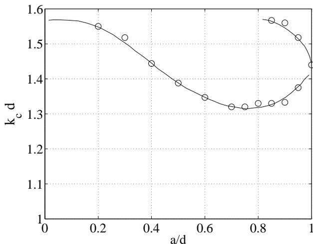
Fig. 7: Resonance frequencies  $k_c d$  as a function of  $a/d$ . Open circles are the experimental values deduced from the resonance curves and plain lines are the theoretical predictions from [20, 21].
