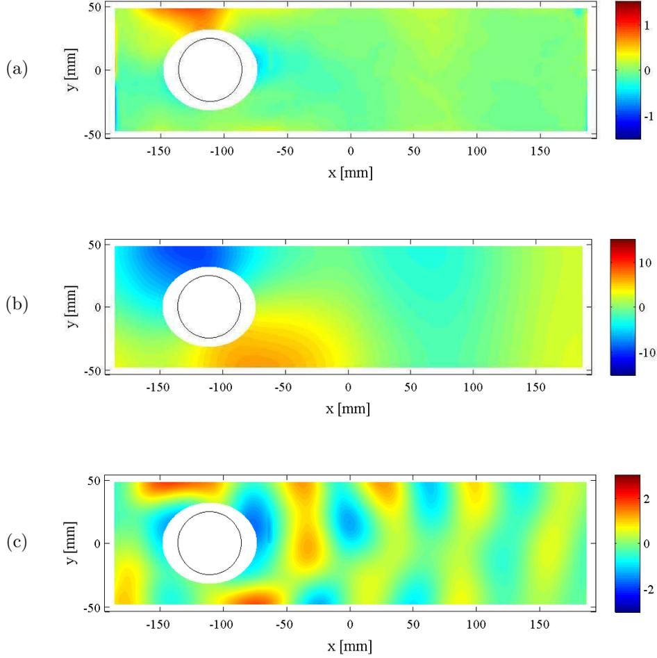
Figure 6: Experimentally measured free-surface deformation fields decomposed in harmonics of the driving frequency: Type I configuration for  $a/d = 0.5$ . (a) Zeroth order contribution  $h_0(x, y)$ , (b) linear contribution  $h_1(x, y, t)$  and (c) first harmonic component  $h_2(x, y, t)$  corresponding to a pulsating frequency of  $2\omega$ . The position of the obstacle within the waveguide is indicated by the black circle. The scale of the colorbar is in mm.
