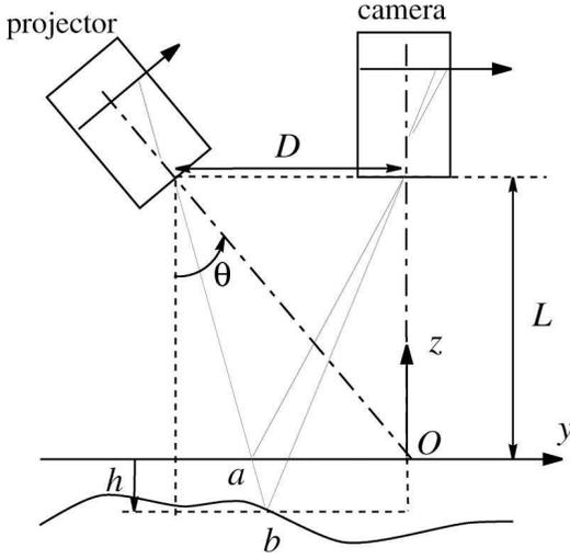
Fig. 1. Reproduction of Takeda's representation in crossed-optical-axes geometry. A fringe pattern is projected onto a reference surface (as point  $a$ ) and on a deformed surface (point  $b$ ). The corresponding phase variation in the intensity recorded by the camera is  $\Delta\varphi(y)$  (2D object analysis is presented in Takeda's paper [2]).
