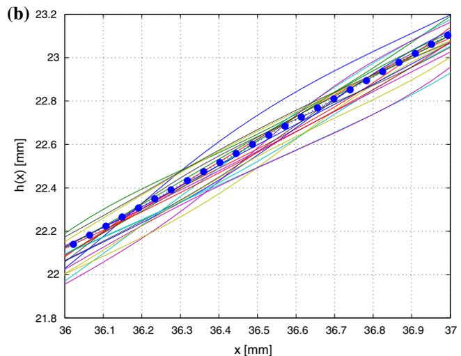
**Fig. 5** **a** Several height profiles measured for the triangular prism used for laboratory testing. **b** Zoom over a portion of the reconstructed profiles showing the precision of the method. In both cases, *dots* indicate the object's profile measured by a 25- $\mu\text{m}$  resolution (point) laser displacement sensor, whereas continuous lines
