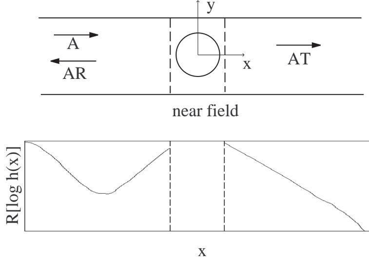
Figure 14: Top: The problem reduces to a 1D problem along the  $x$ -axis, by projecting the antisymmetric field onto the first transverse mode in  $\sin \pi y/2d$  outside the near field region. Bottom: Typical variation of  $h(x)$  along the  $x$ -axis: real part of  $\log[h(x)]$  as a function of  $x$  (a.u.) (the curve has been obtained for  $a/d = 0.4$ ,  $kd = 1.47$ ).
