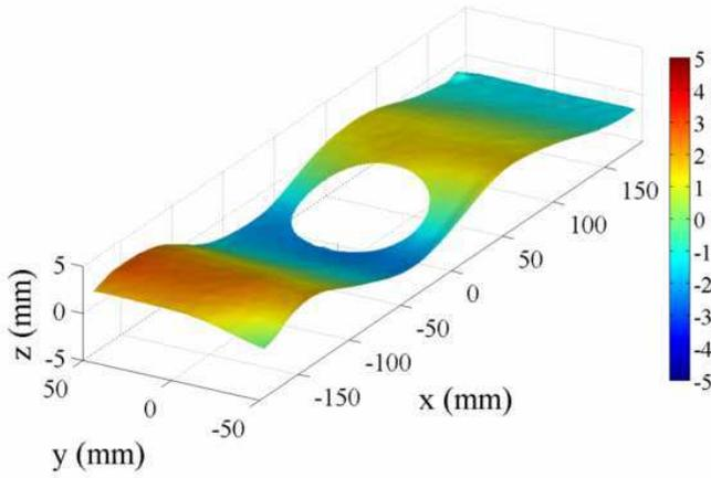
Fig. 2: Typical instantaneous fields of the surface elevation  $h_T(x, y, t)$ , here for  $a/d = 0.50$ ,  $kd = 1.32$ . The scale of the colorbar is in mm.
