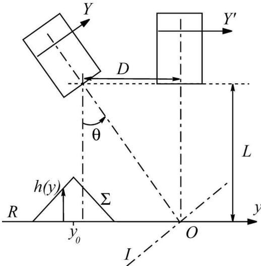
Fig. 5. Experimental configuration:  $\Sigma$  is at distance  $h(y)$  from the reference plane  $R$  with  $h(0 < y - y_0 \leq -3 \text{ cm}) = y$ ,  $h(0 < y - y_0 \leq 3 \text{ cm}) = -y$  zero, otherwise.  $I$  is the image plane of the projector. In the experiments,  $L = 105.2 \text{ cm}$  and  $\theta$  can vary, and for  $\theta = 0^\circ$  (parallel-optical-axes geometry),  $D = 18 \text{ cm}$ .
