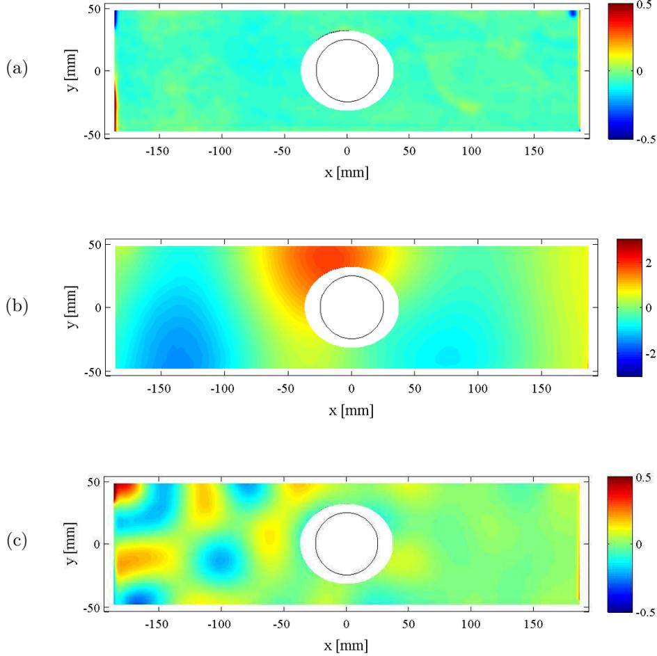
Figure 7: Experimentally measured free-surface deformation fields decomposed in harmonics of the driving frequency: Type II configuration for  $a/d = 0.5$ . (a) Zeroth order contribution  $h_0(x, y)$ , (b) linear contribution  $h_1(x, y, t)$  and (c) first harmonic component  $h_2(x, y, t)$  corresponding to a pulsating frequency of  $2\omega$ . The position of the obstacle within the waveguide is indicated by the black circle. The scale of the colorbar is in mm.
